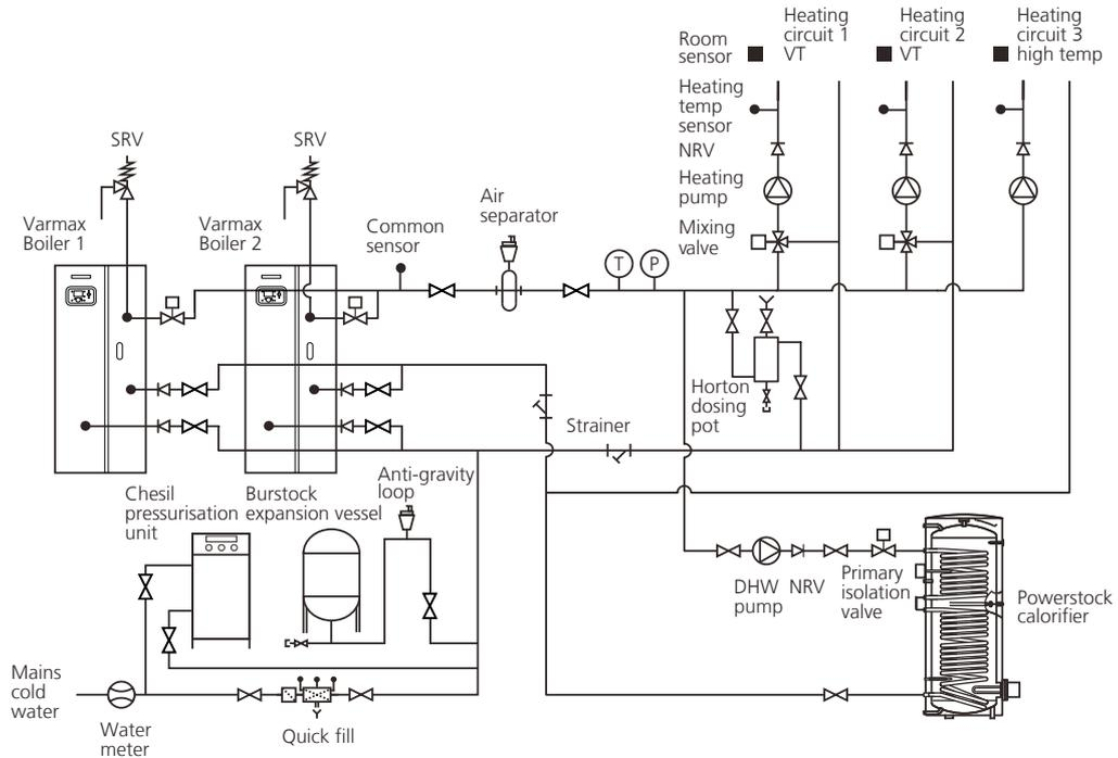
**Scheme 4: Multiple boilers with low loss header**
