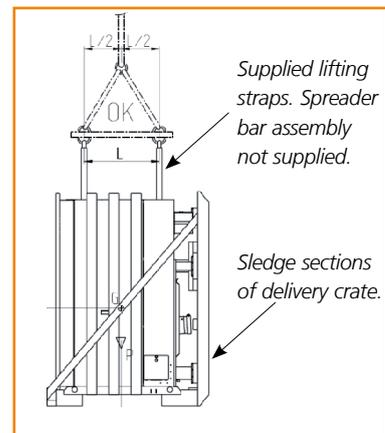
Every boiler is supplied with lifting eyes on top of the heat exchanger to which straps are factory fitted and correctly located for crane lifts to elevated boiler house locations. A suitable spreader bar must be used when lifting the boiler using the supplied straps to protect the casings and components on top of the boiler.
