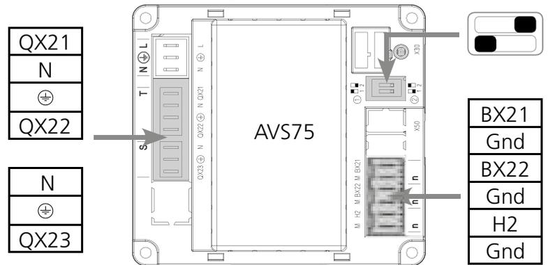
The heating circuit control kit has the ability to manage control of the heating circuit pump, mixing valve and receive a feedback signal from a flow temperature sensor within the circuit.
