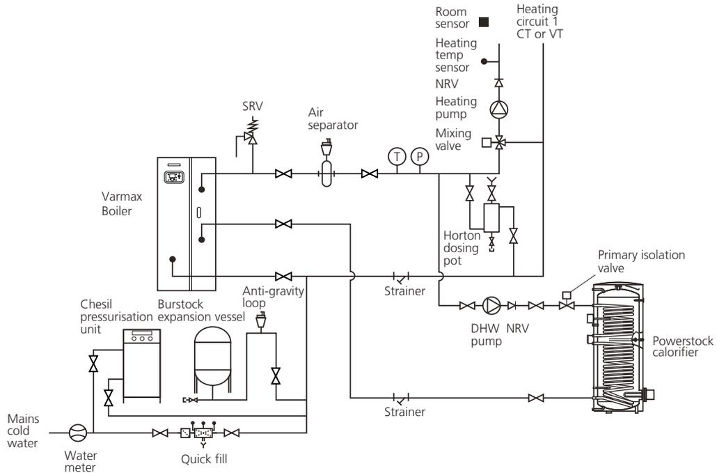
**Scheme 2:** Single boiler with multiple split temperature heating circuits and domestic hot water
