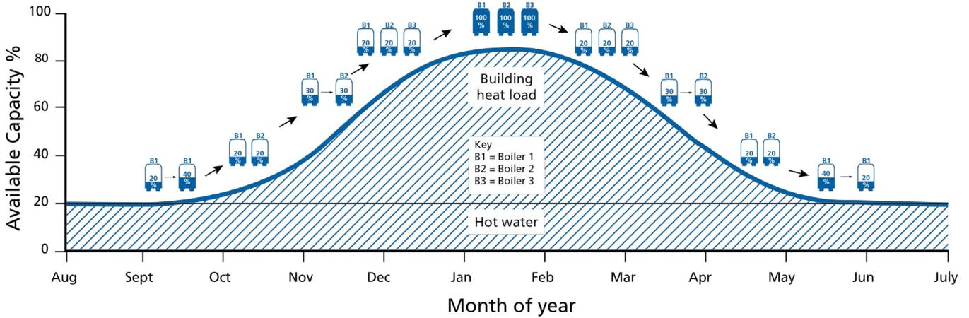
The overall efficiency of a multiple boiler plant depends on how close its total output can be controlled to match the load profile of the building. Therefore, it is a really important aspect of product selection.
