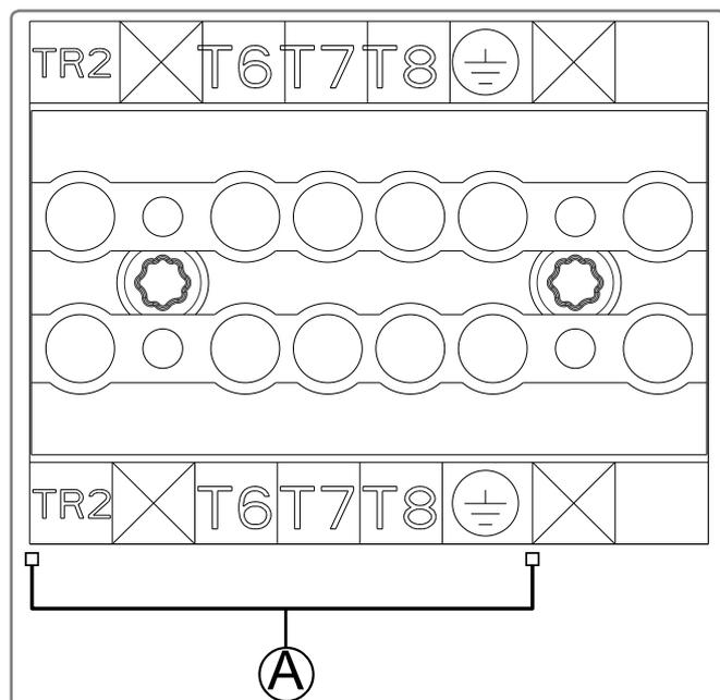
figure 21 - Connection of the cable to enable operation of the burner's second stage
