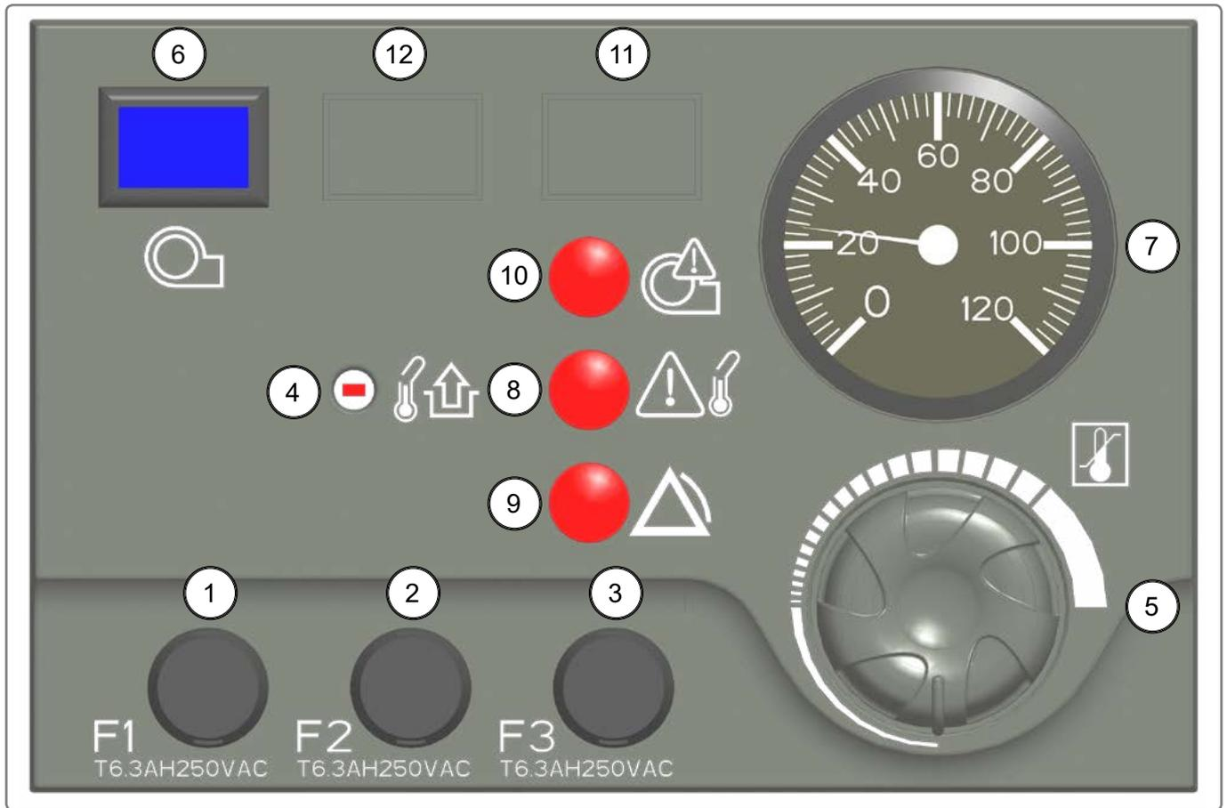
figure 2 - Thermostat module
