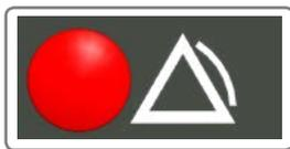
If the external safety interlock circuit LED is lit up, refer to the external appliance which is connected to terminals 3, 4 and 5 of the control panel to identify the fault, find the cause and eliminate it. It is not necessary to reset the control panel.
