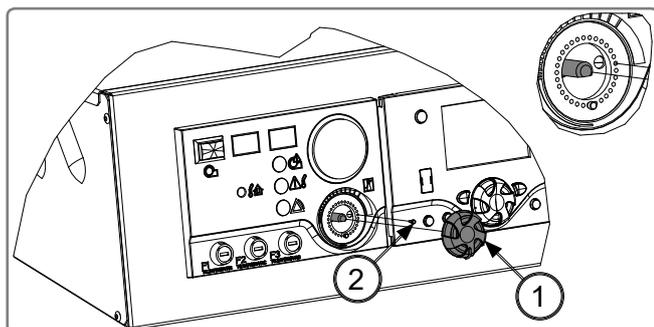
figure 26 - Positioning the thumbwheel's stopping pin
