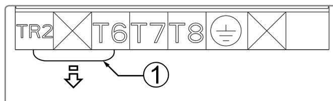
figure 22 - Removal of shunt
