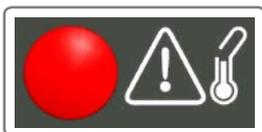
If the overheat LED is lit up, find the cause of overheat and repair if necessary. Once the problem has been solved, it is necessary to manually reset on the safety thermostat.
