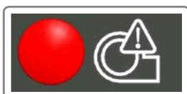
If the burner fault LED is lit up, refer to the burner documentation to identify the fault, find the cause and eliminate it. It is not necessary to reset the control panel.
