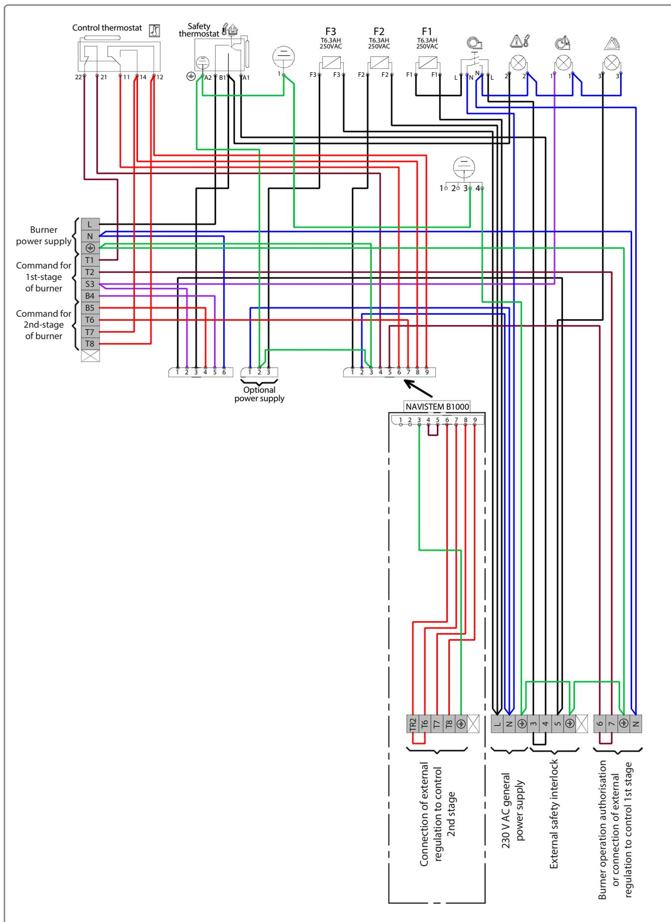
figure 15 - Control panel electrical connection diagram
