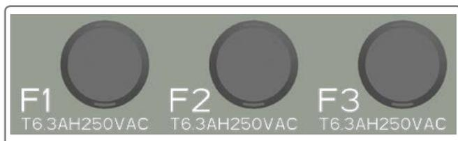
figure 29 - Position of fuses
