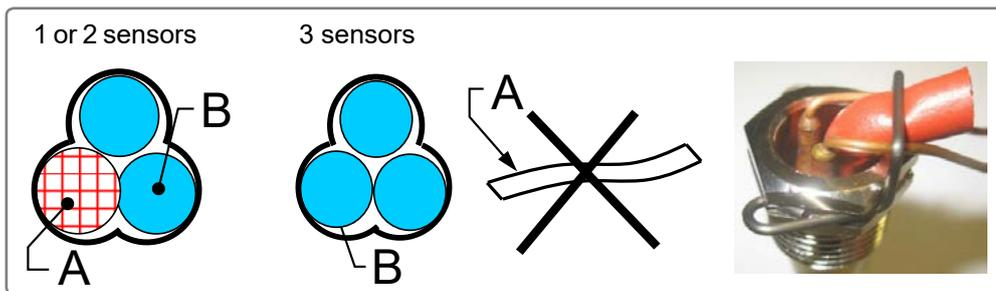
figure 9 - Installation of sensors
