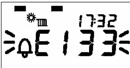
Fig 7.3.3 - Boiler Display With Low Inlet Gas Pressure
