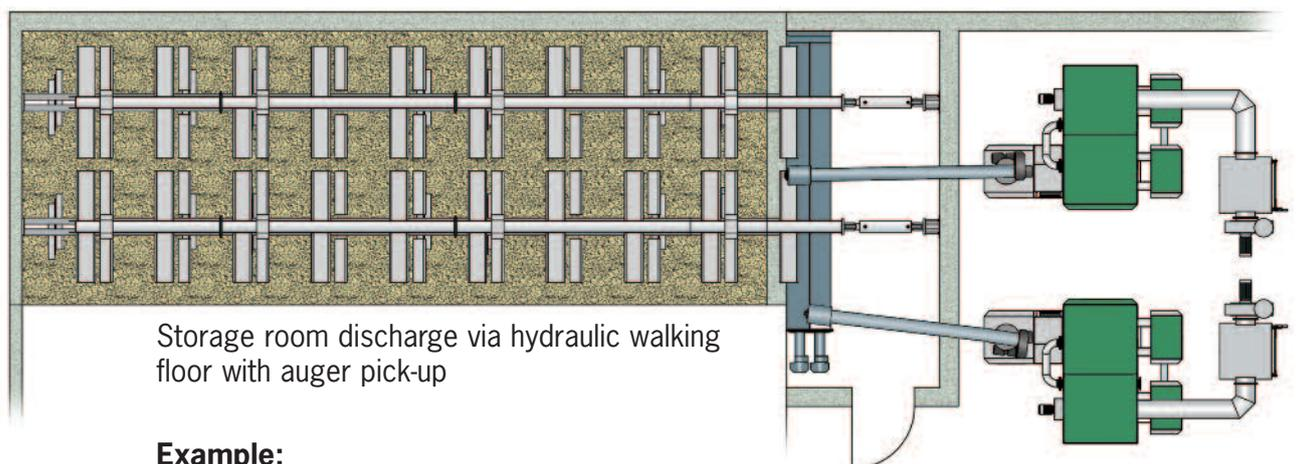
Storage room discharge via hydraulic walking floor with auger pick-up
