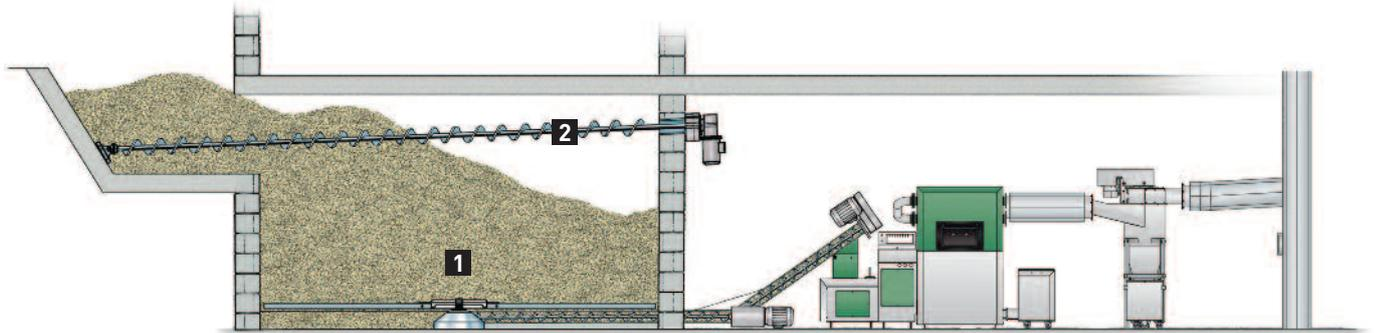
Storage room discharge via horizontal spring agitator (1) with rising screw allows optimum usage of the fuel storage room. The filling screw (2) distributes chip evenly during delivery
