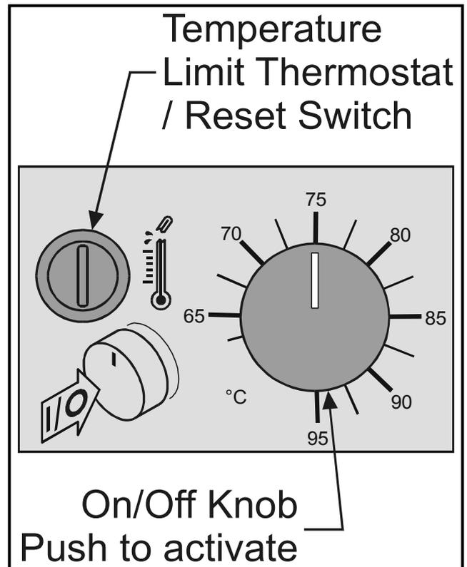
110°C. The minimum difference between control thermostat and temperature limiter **MUST NOT** be less than 10°C.
