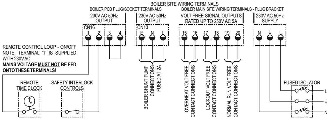
2) MULTIPLE BOILER INSTALLATION, ON/OFF OR HIGH/LOW (CLASSIC WITH FLUE HIGH/LOW FLUE DAMPER MODELS ONLY) OPERATION VIA HAMWORTHY HEATING LIMITED MILTON BOILER SEQUENCE CONTROL. NOTE: ROTARY SWITCH 'SW1' ON THE SEQUENCING INTERFACE MODULE - POSITIONS '1' TO '9' SETS THE BOILER FIRING ORDER.
