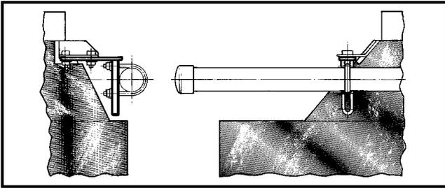
Figure No. 10.3c shows the pipe clamp fitted to Purewell 40, 50, 95 and 105 kW boilers.
