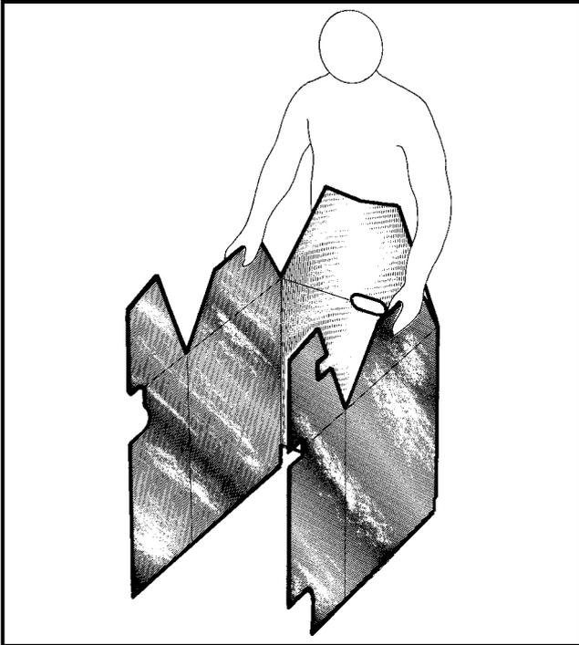
Reference to Figure 10.2b - Insulation should be folded around boiler such that its rear edges meet in the centre. Ensure flow and return connections are clear and unobstructed. Apply foil tape down join.
