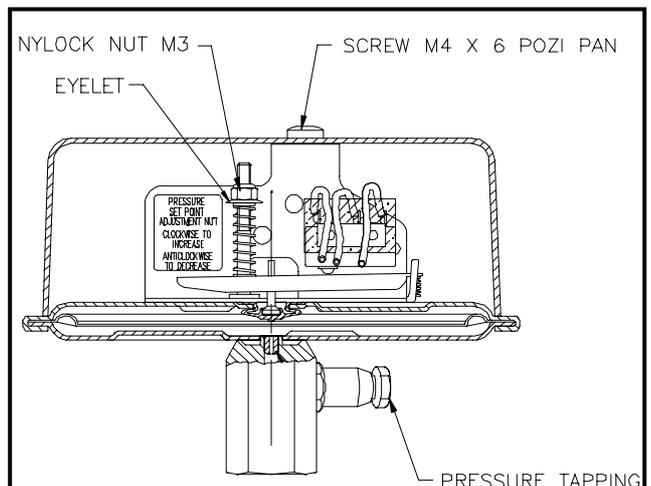
With the cover removed, turn the M3 nut clockwise to increase the set point and vice-versa. Seal the adjuster after setting.
