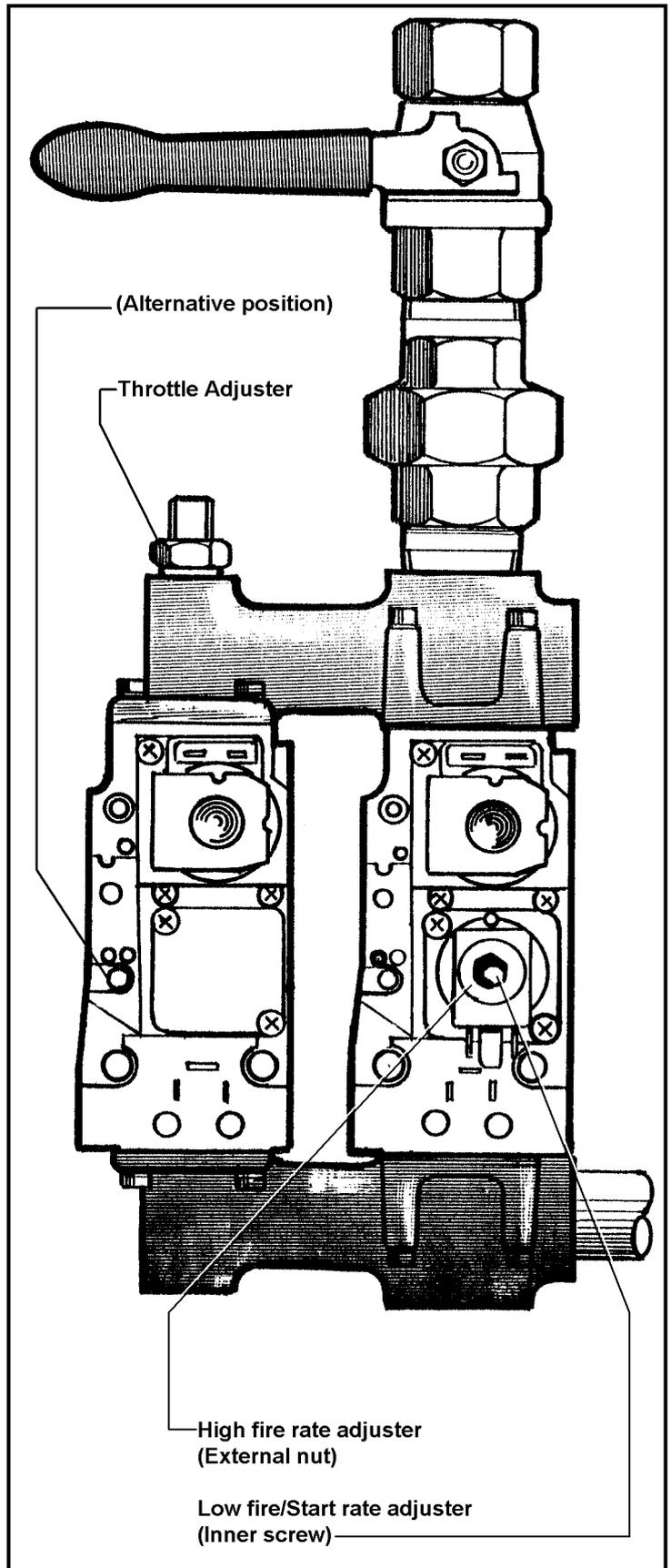
valve system up to high fire. Check gas pressure against that shown in Figure 2.2 (p4) or Appendix 'A' (p37). If necessary adjust high fire governor to suit. Occasionally this high fire adjustment can influence the low fire (start rate), therefore remove link and check low fire pressure again. Adjust if required. Repeat until low and high fire pressures are as shown in Figure 2.2 (p4) or Appendix 'A' (p37).
