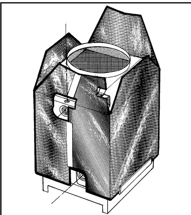
Reference to Figure 10.2c - Fold down petals as shown. Use foil tape to affix edges. Fold as required. Ensure gas pipe bracket is clear and unobstructed.
