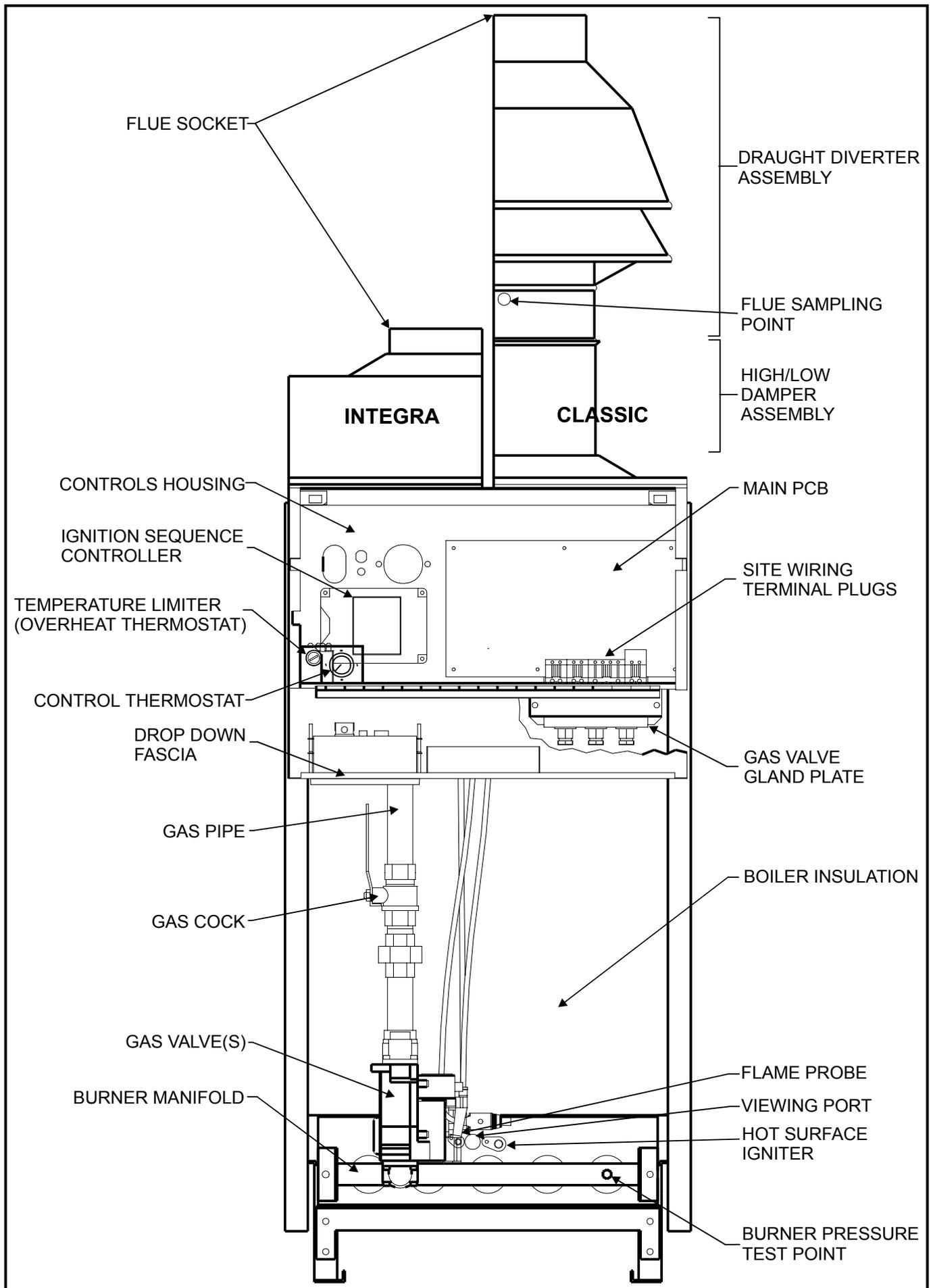
Figure 14.1 Diagram of Hot Surface Igniter and Sensing Probe Assembly
