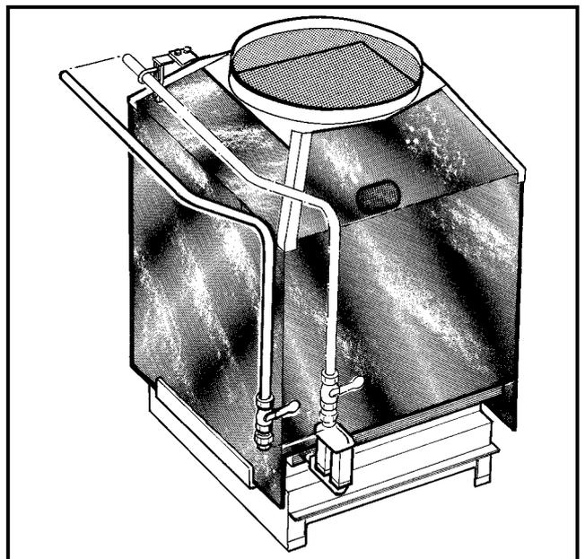
Figure No. 10.3b shows the pipe clamp fitted to Purewell 60, 70, 80 and 120 kW boilers.
