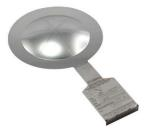
Burst Discs consist of a thin membrane which is designed to break and open when the specific level of differential pressure rises above the resistance limit that the disc was originally calibrated for, so as to allow for the excess pressure to vent out safely.
