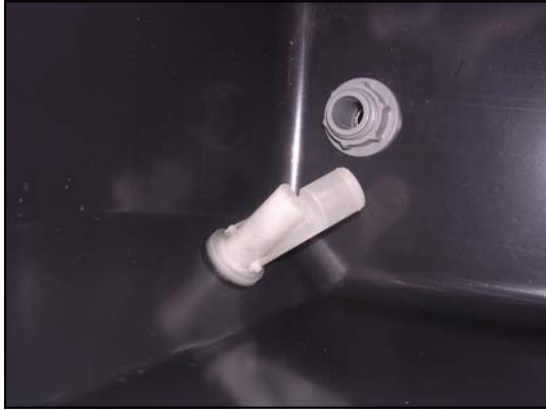
Figure 31 - Level Switch In Tank
