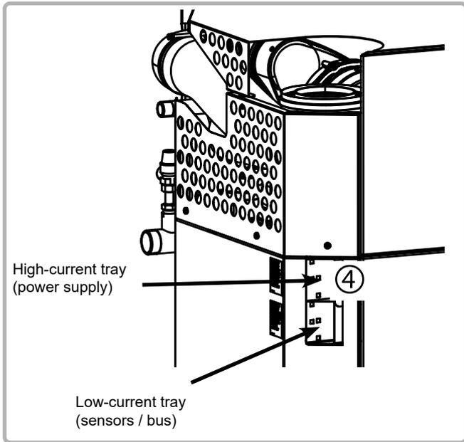
figure 17 - Electrical cable duct
