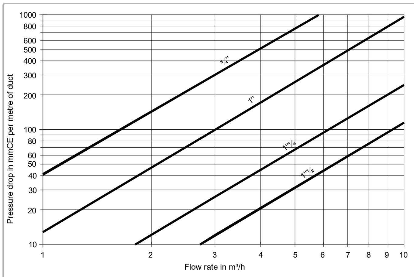
figure 11 - Diagram of regular pressure drops in steel ducts (cold water)
