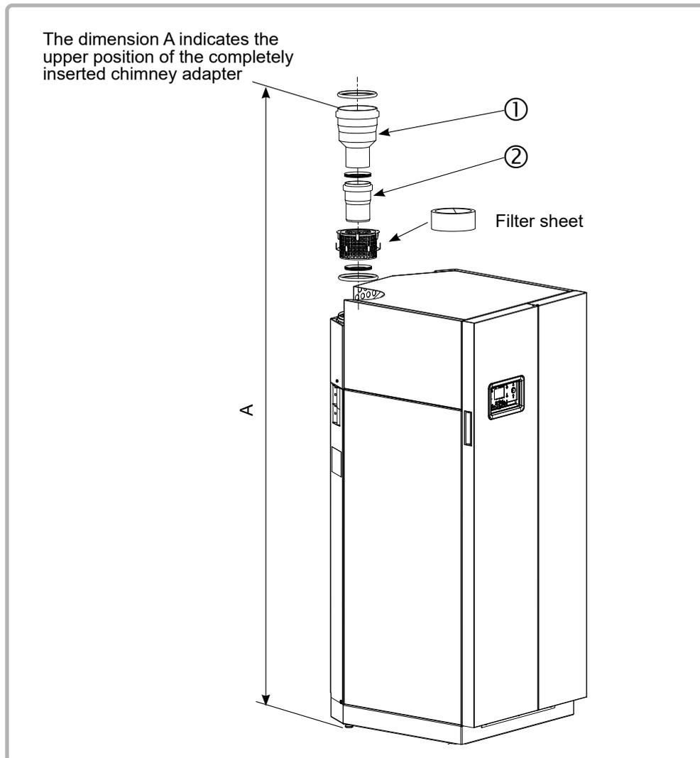
figure 5 - Connection to a chimney
