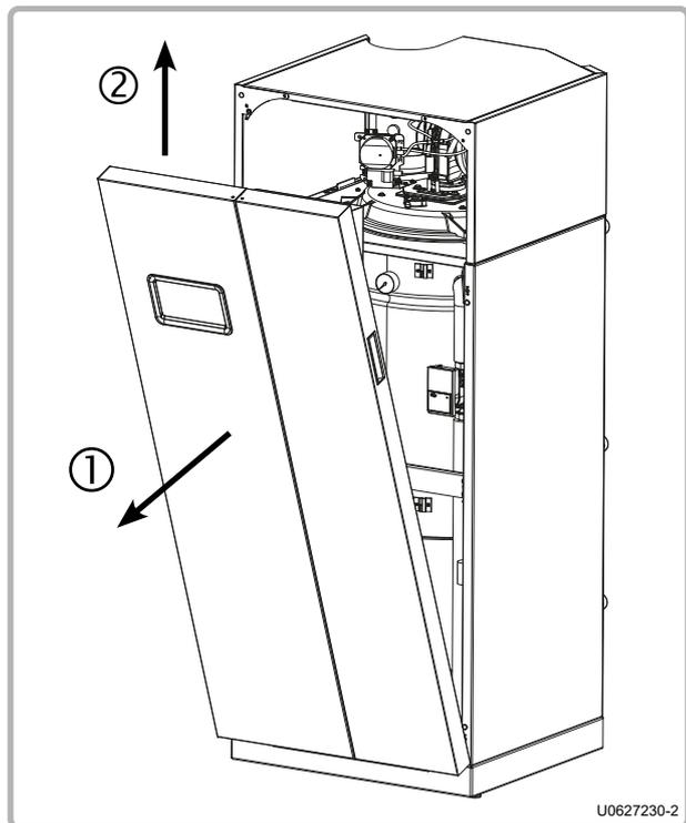
figure 3 - Removing the front panel
