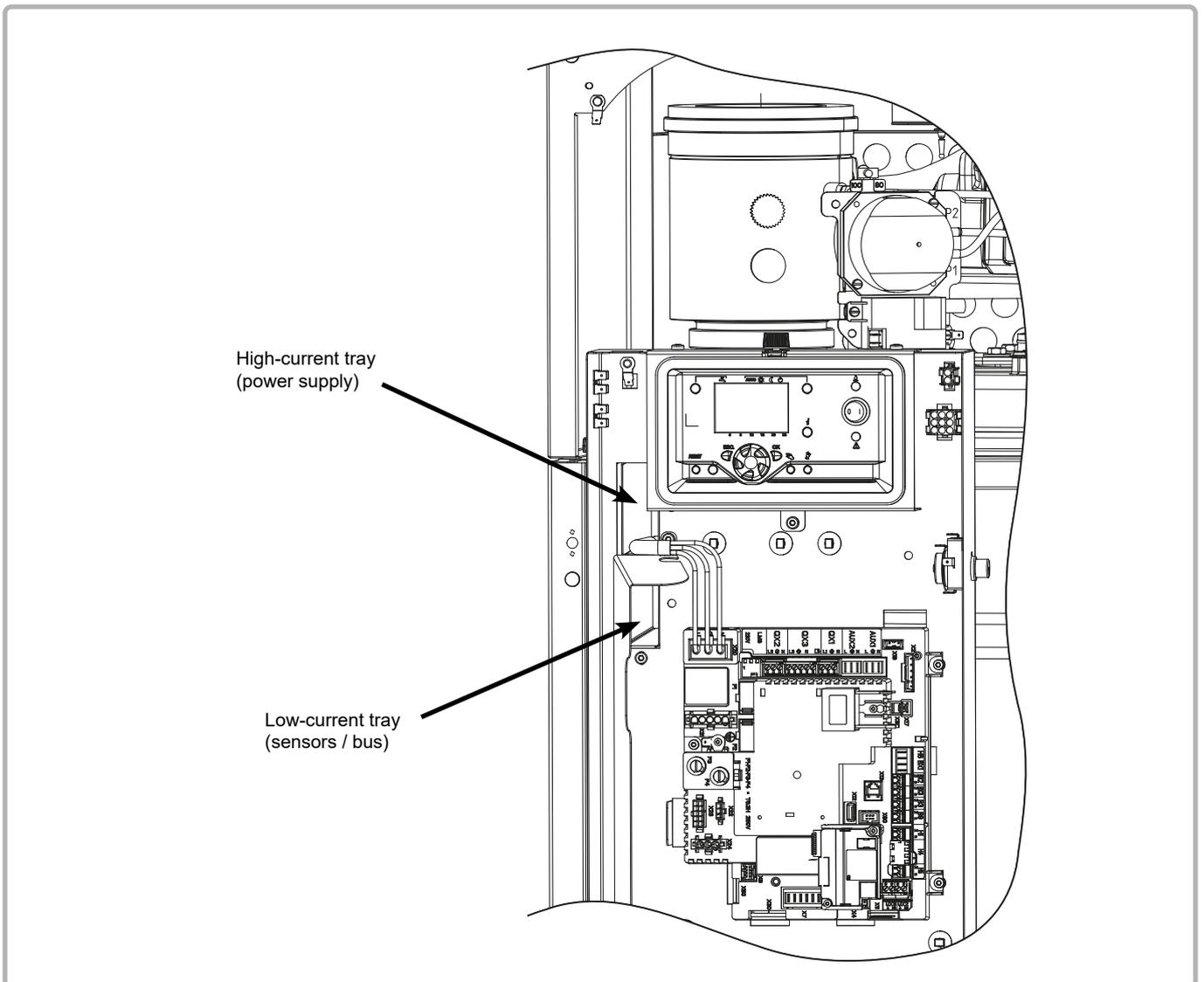
figure 18 - Electrical cable duct
