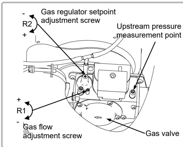
figure 14 - R1 and R2 adjustment screws
