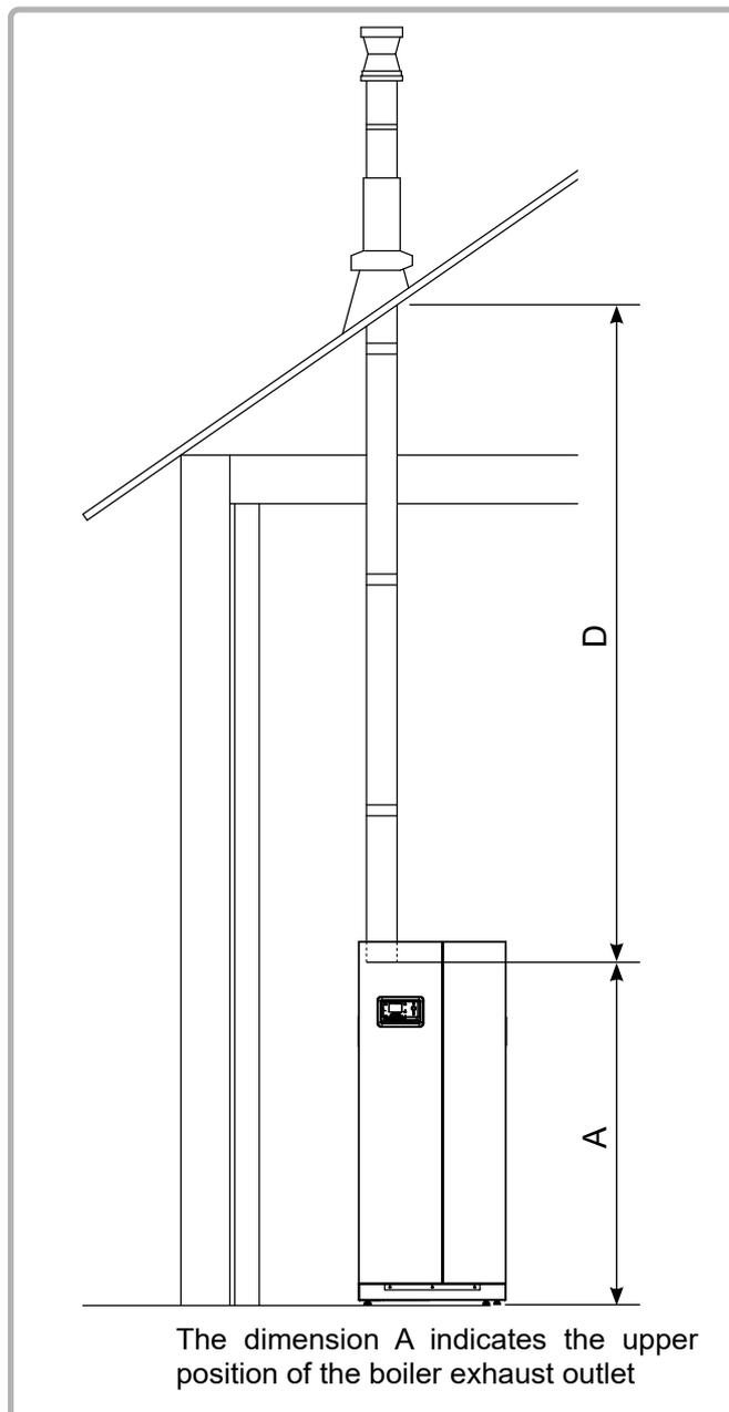
The dimension A indicates the upper position of the boiler exhaust outlet
