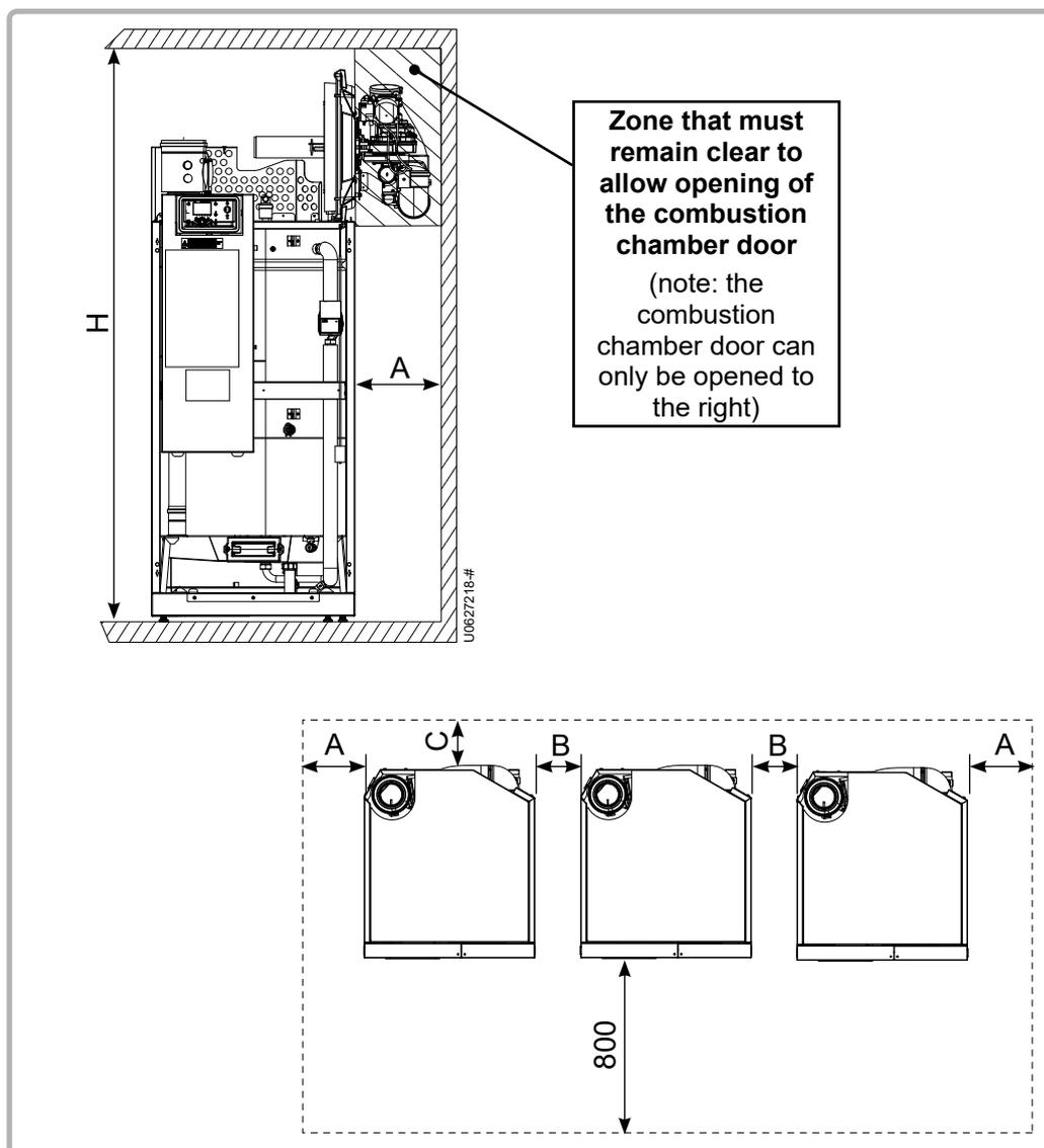
figure 2 - Clearance around the boiler
