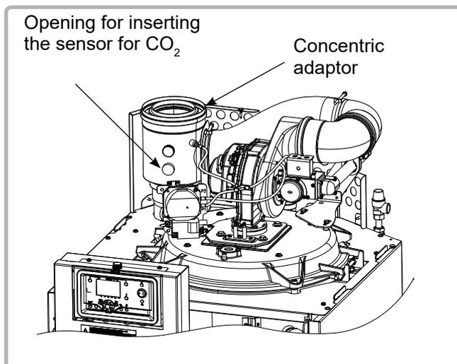
figure 15 - Measurement orifice
