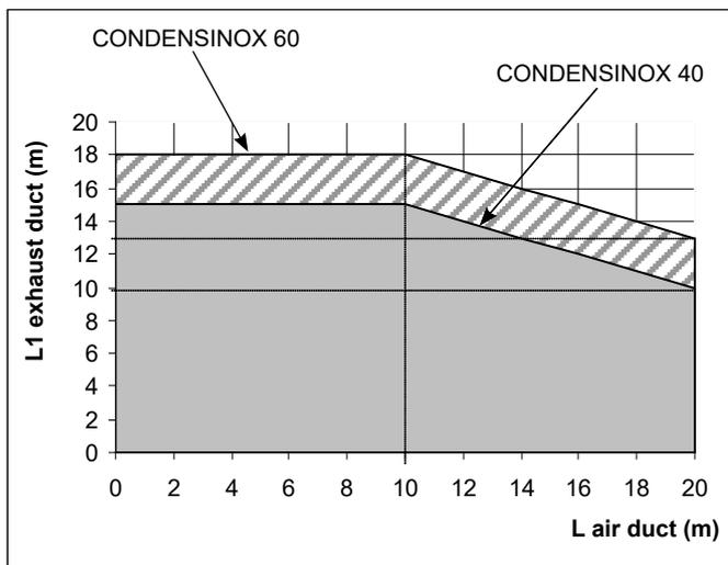
figure 9 - Max length of C53 type ducts
