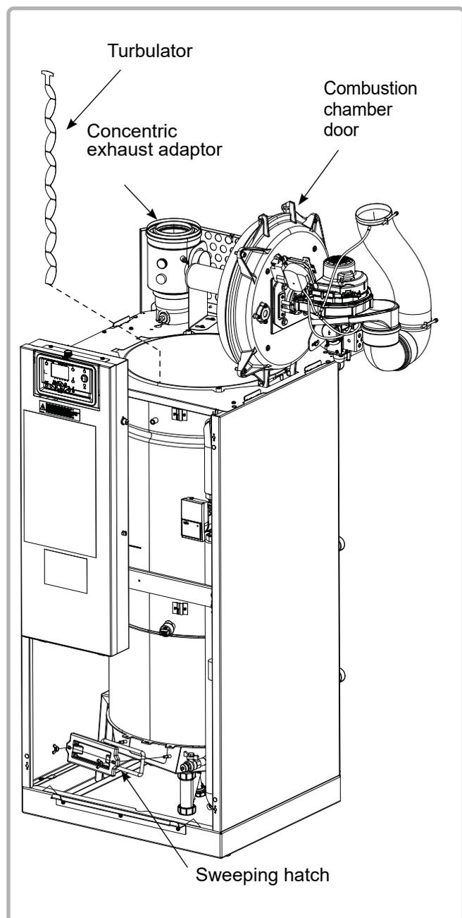
figure 20 - Cleaning the combustion chamber/exchanger
