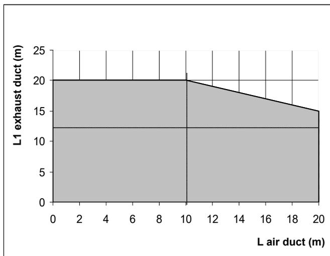
figure 10 - Max length of C53 type ducts
