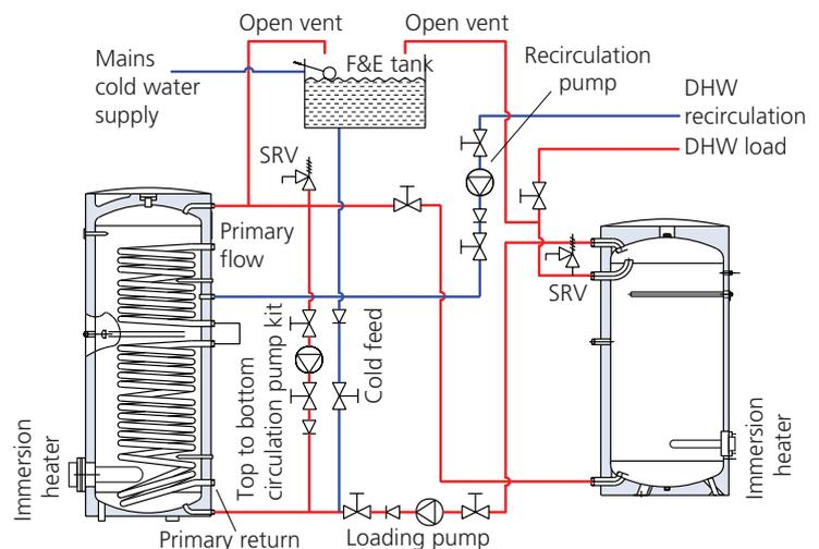
\*The immersion heater can only be used with models PS300 to PS1000.
