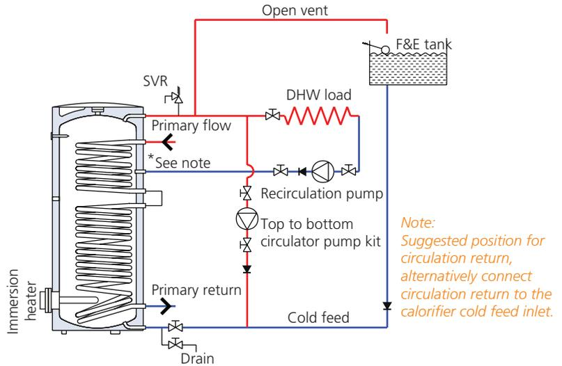
*Note:* Suggested position for circulation return, alternatively connect circulation return to the calorifier cold feed inlet.
