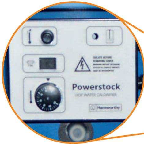
A control panel is provided for each cylinder housing a control thermostat, with a range 0°C to 120°C, pre-set at 60°C, and a high limit thermostat pre-set at 85°C, non-adjustable.
