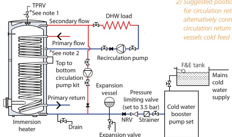
\*The immersion heater can only be used with models PS300 to PS1000 in this configuration.
