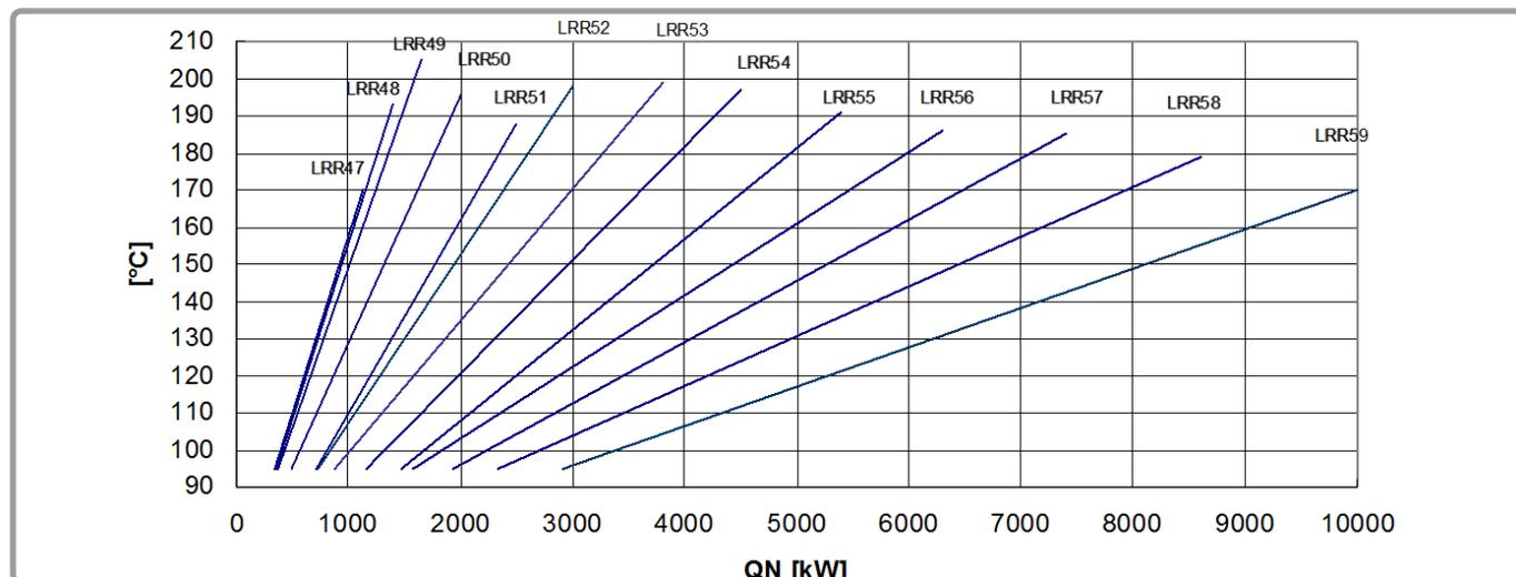
figure 8 - Flue gas temperature diagram LRR, natural gas with clean boiler
