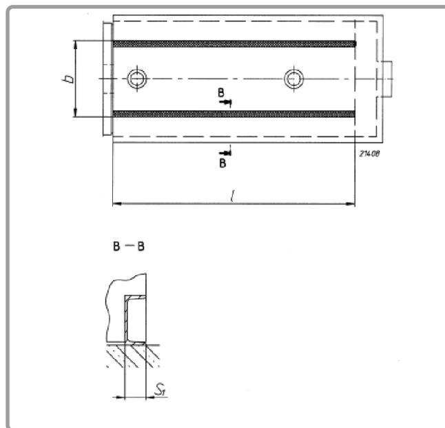
figure 14 - Without vibration dampers
