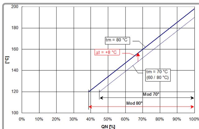
figure 11 - Flue gas temperature – Boiler power diagram (example for two average boiler water temperatures)
