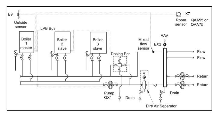
Figure E 1.3.3 - Schematic 3 - Master and Slave Sequence Control With Reverse Return Primary
