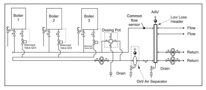
Figure E 1.3.6 - Schematic 6 - Reverse Return Primary Circuit with Individual Motorised Boiler Isolation
