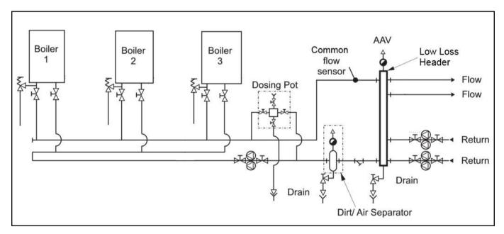
Figure E 1.3.4 - Schematic 4 - Reverse Return Primary Circuit
