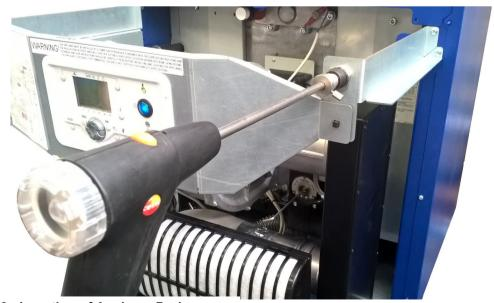
Figure 8.5.2 - Insertion of Analyser Probe
