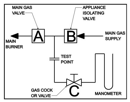
Figure 7.1 - Gas System Leak Check Diagram
