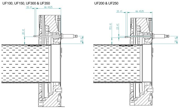
Figure 10.2.1 - Spark Electrode position
