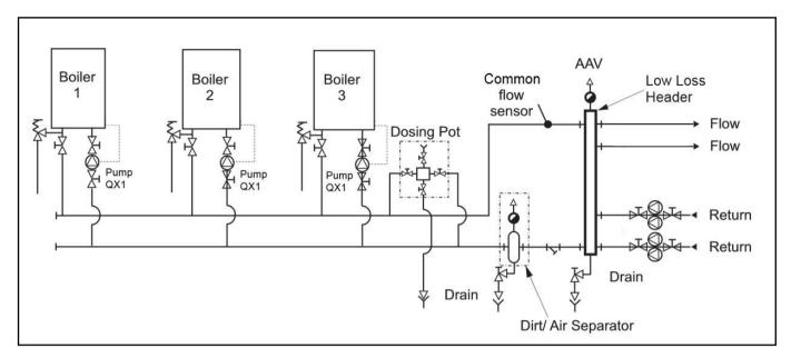
Figure E 1.3.5 - Schematic 5 - Primary Circuit With Individual Boiler Shunt Pumps
