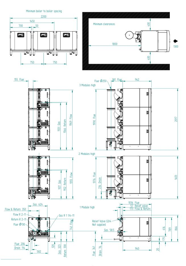
Figure 3.1.3 - Dimensions and Clearances UF300 & 350
