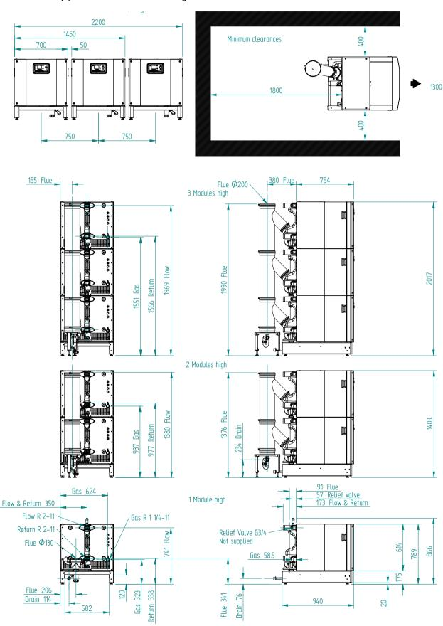
Figure 3.1.1 - Dimensions and Clearances UF100 & 150
