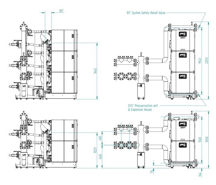
Figure 3.2.2 - UF100 & UF150 2MW Primary circuit and Gas manifold pipe kit
