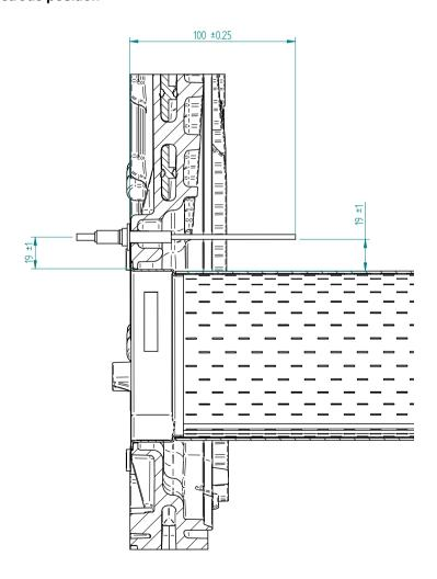
Figure 10.2.2 - Flame Probe position
