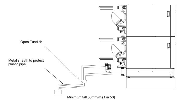
Figure 4.5.1 - Boiler Condensate Connection
