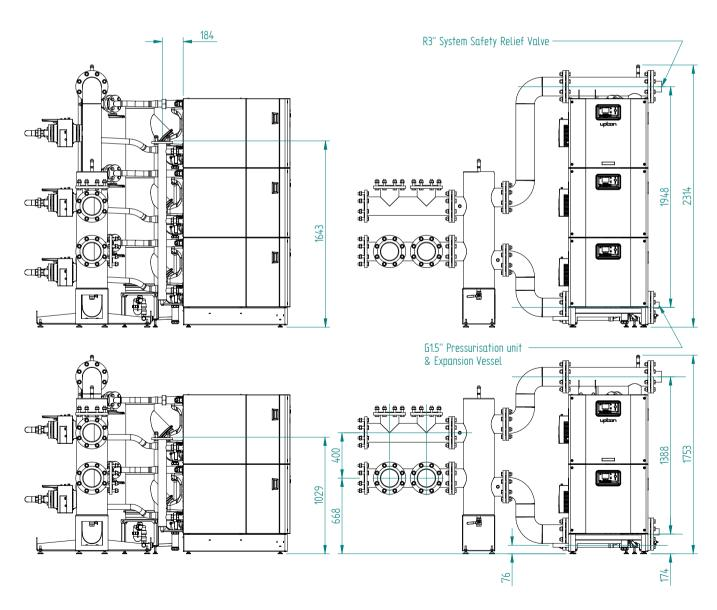
Figure 3.2.3 - UF200 & UF250 3MW Primary circuit and Gas manifold pipe kit
