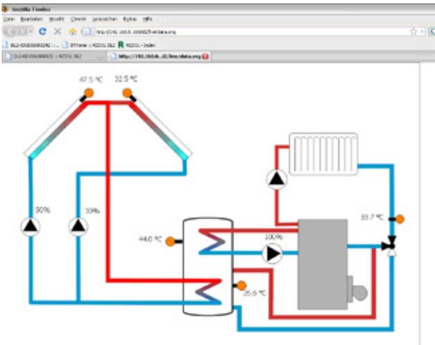
Live data can also be displayed in a graphical system scheme in the web interface.
