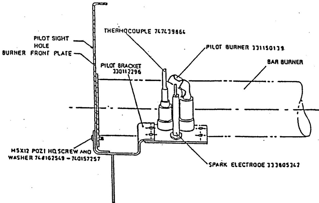
PILOT BURNER ASSEMBLY ( PERMANENT PILOT ) fig.13 a
