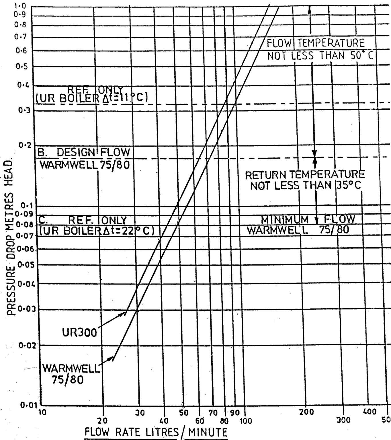
If flow rate between 'B' and 'C', the system RETURN temperature under normal operating conditions may be down to  $35^\circ\text{C}$ .
