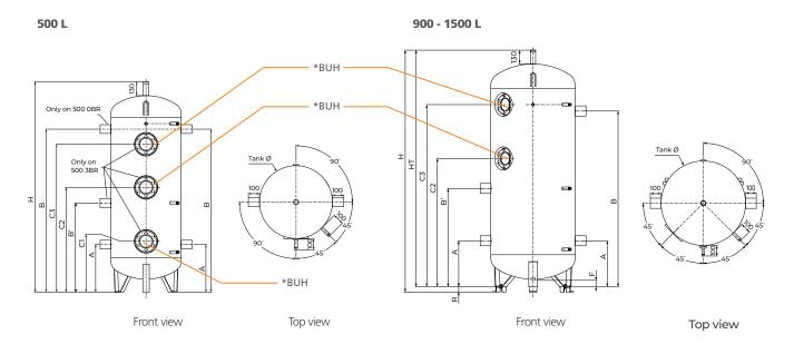
\*BUH - Back up heater mounting points only, must not be used for water flow / return connections.
