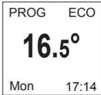
If the screen displays ECO PROG, you are in a programming range in ECO mode.
