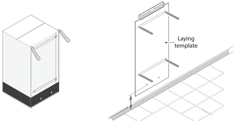
Drill and plug the water heater and use attachments of at least 10 mm in diameter ( $\varnothing$ ) suitable for your wall type (drywall, concrete, brick).
