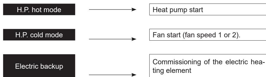
In test mode, heat mode heat pump starts, 3 minutes after power-up, only if the following conditions are met:
