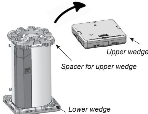
The suspended device's upper wedge consists of 2 parts: the spacer serves to protect the connection ports and the lower cover when the water heater has been turned.
