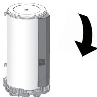
The suspended device can be turned when it has been moved towards the bearing wall.
