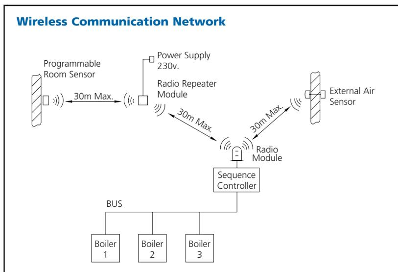
The repeater module requires a dedicated power supply and is supplied with a plug in transformer 230v – 7.5v with 3 metre cable to supply power to the repeater. A switched mains socket outlet is required within 3 metres of every repeater.
