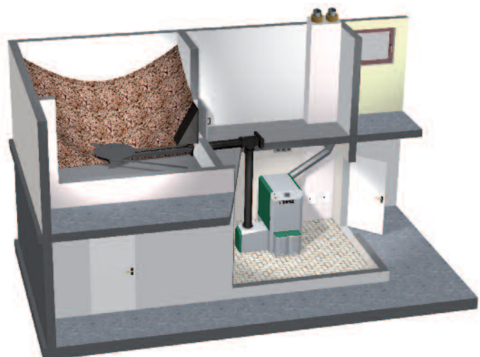
Storage room and boiler room at different levels. Horizontal discharge with spring agitator and chute pipe.
