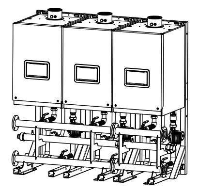
All headers and pipe work should be insulated in accordance with the Non Domestic Building Services Compliance Guide. To ensure compliance with the maximum heat loss criteria, insulation thickness should be calculated according to BS EN ISO 12241 using standardised assumptions.
