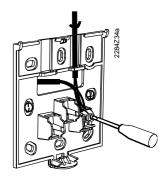
Engage the housing front at the top of the base and close the unit to the bottom.
