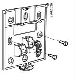
Pull the interface cable through the opening of the base and connect it to the screw terminals.
