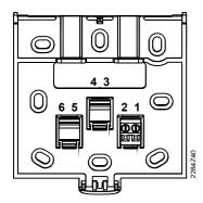
1 COAOpen Therm terminal A (interchangeable)2 COBOpen Therm terminal B (interchangeable)3 --4 --
