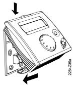
Slide the unit into the panel cut-out without applying any force.
