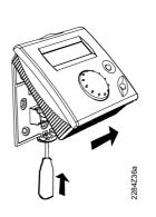
Fit the base to the wall with screws.
