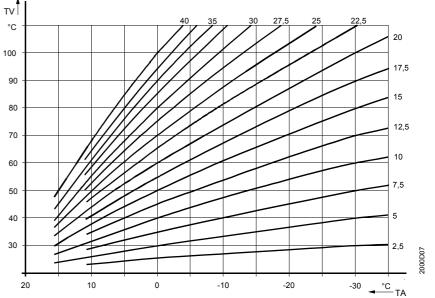
TV = Flow Temperature, TA = Composite Outside Temperature, Factory Setting = 15 i.e. 1.5:1 ratio. For under-floor heating circuits a maximum curve setting of 8 is recommended to prevent overheating.
