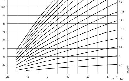
TV = Flow Temperature, TA = Composite Outside Temperature, Factory Setting = 15 i.e. 1.5:1 ratio.
