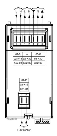
Connect the flow sensor, QAL36, supplied with the kit, using a twisted pair shielded cable, to terminals X51-01 on the second heating circuit clip-in relay.
