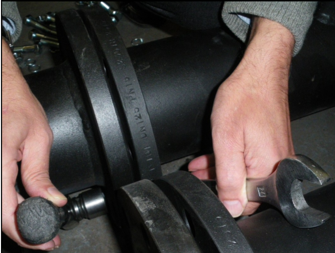
Figure 5.7 - Bolting Method To Assemble Pipe Kit Flanges Together.
