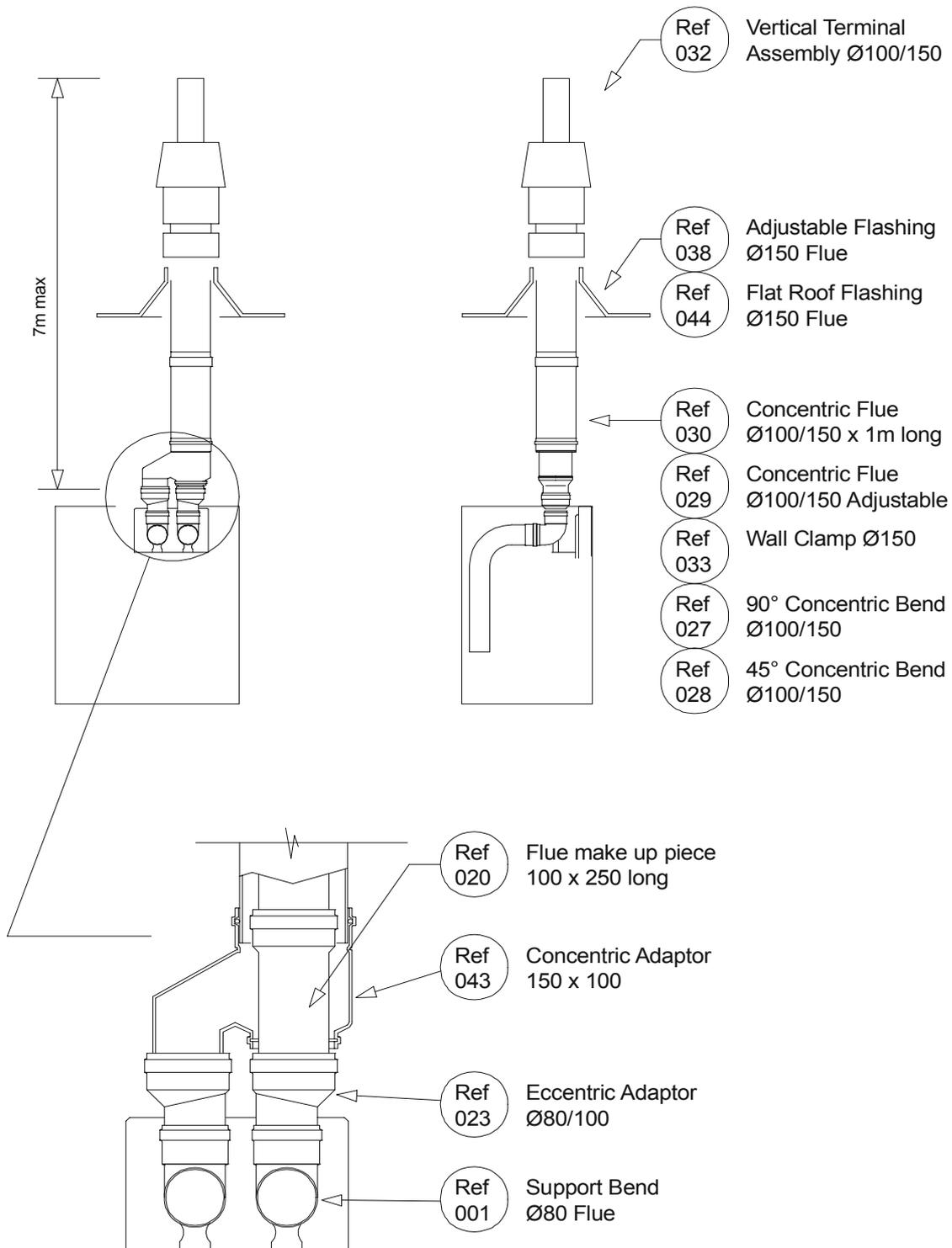
Enlarged detail showing cut section through concentric adaptor
