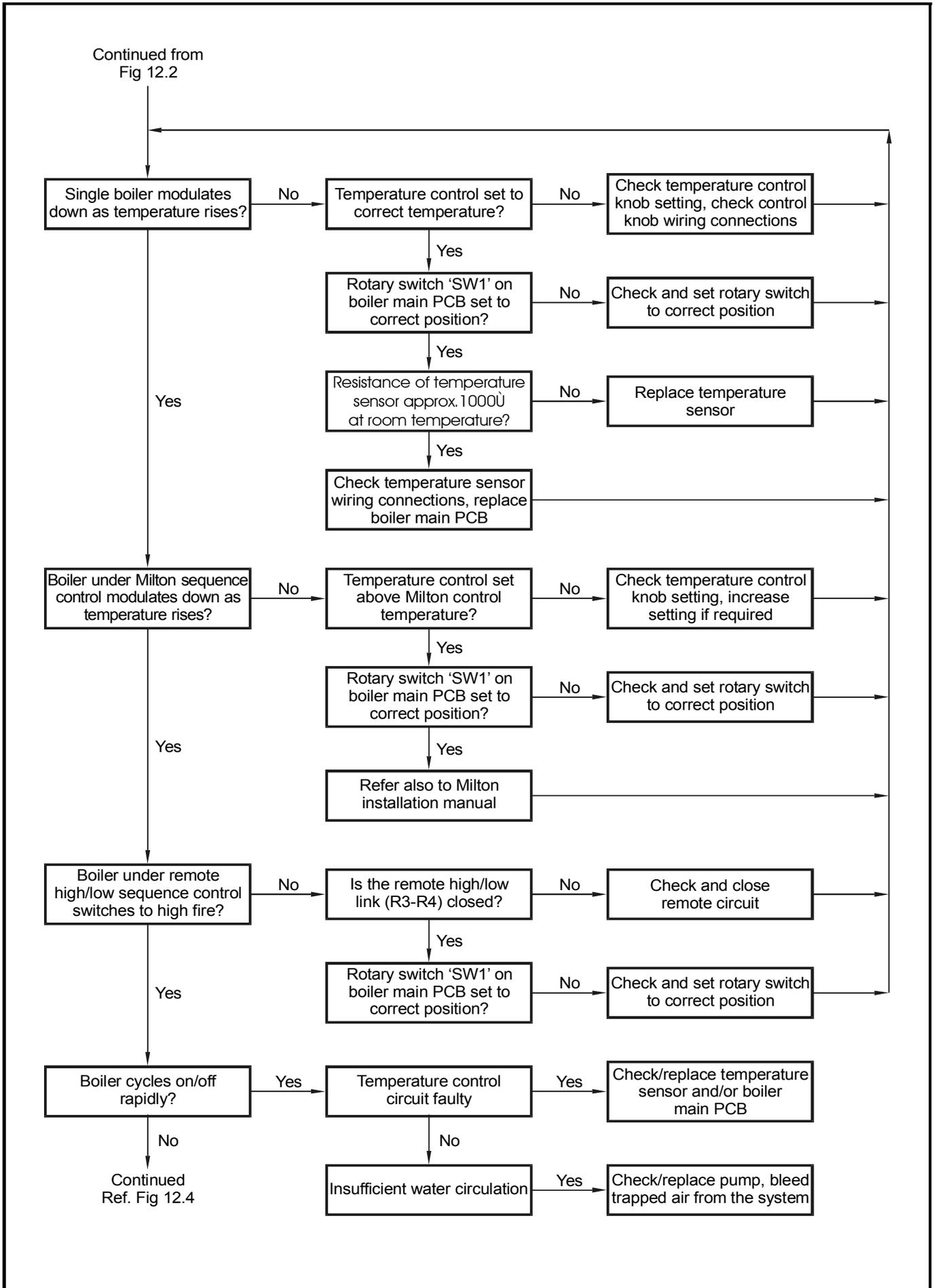
**Figure 12.4. Fault Finding Procedures.**
