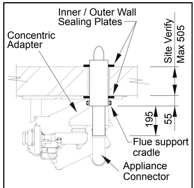
**Figure 10.3.1.1 Connection of Flue System (Concentric Ducts Horizontal) - Frame Mounted Option**
