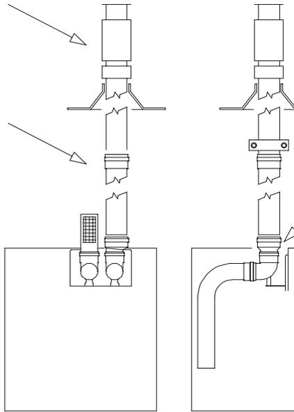
Ref 039 Flat Roof Flashing Ø100 flue
