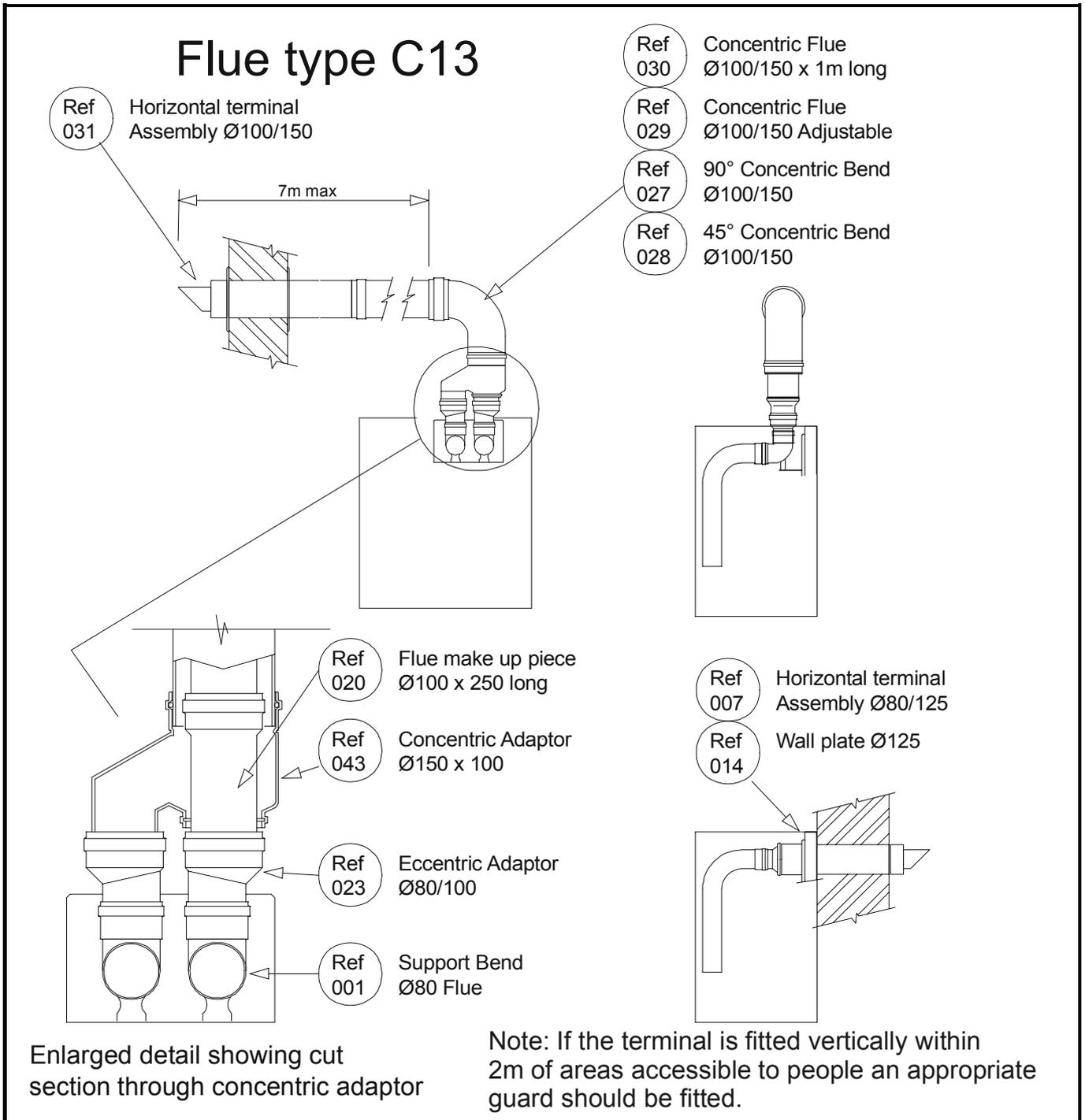
Figure 6.1.2. - Vertical Balanced Flue
