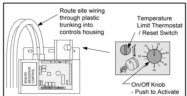
**Figure 8.12 Site Wiring Diagram (Page 1 of 2)**
