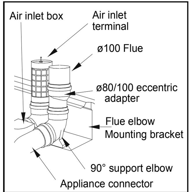
**10.3.4 Connection of Single Pipe Horizontal/ Vertical Open Flue – 100mm**
