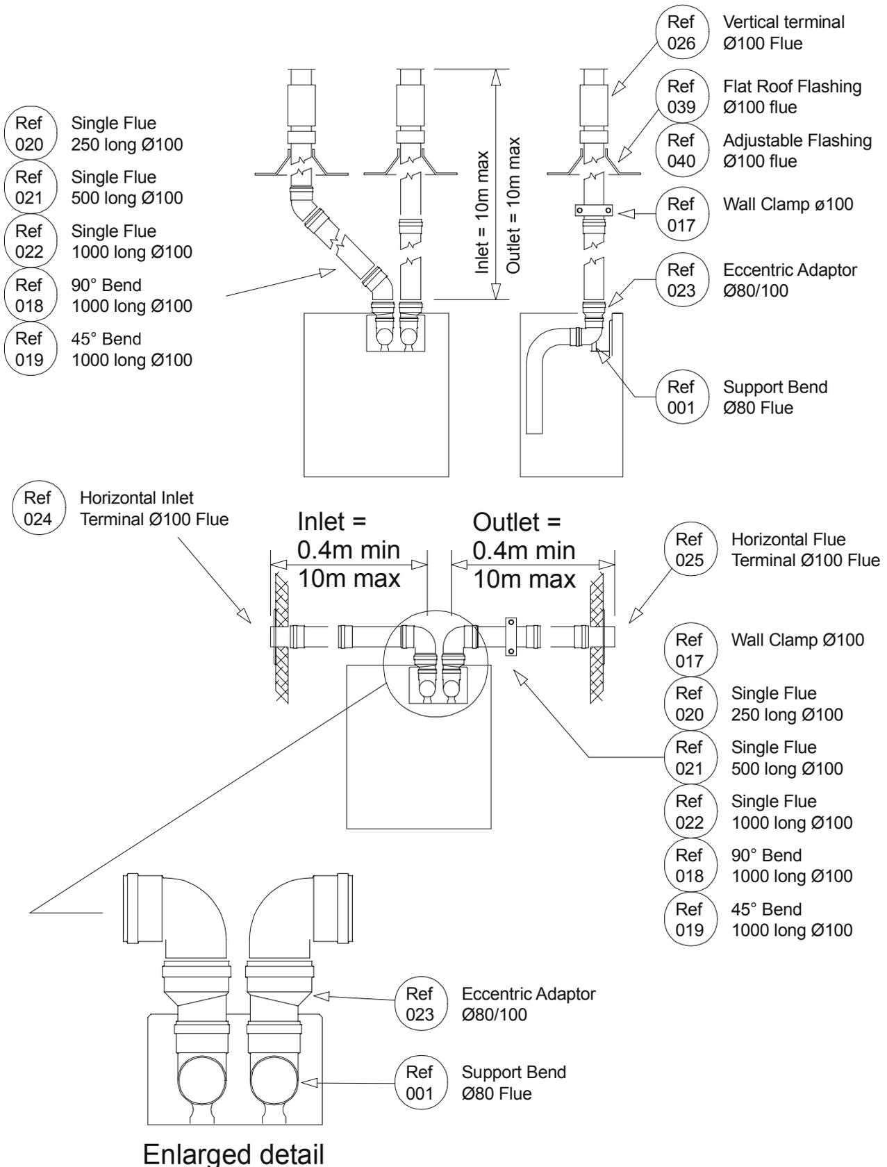
Figure 6.1.4. - Intake from Ventilated Plant Room and Discharge via Horizontal/Vertical Flue
