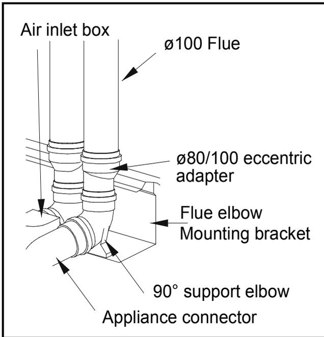
**Figure 10.3.4 Connection of Single Pipe (Open Flue)**
