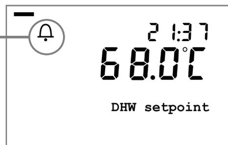
When a fault causes the battery to trip, the fault code and its label are permanently displayed on the screen. Similarly, a small bell appears at the top LH corner of the display.
