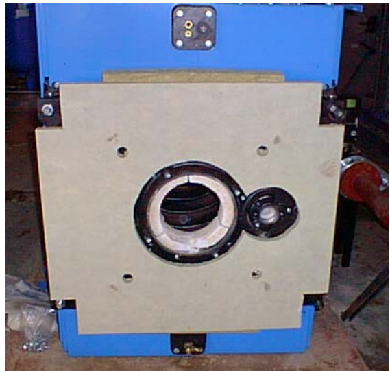
Picture 10: Door Casing Insulation
