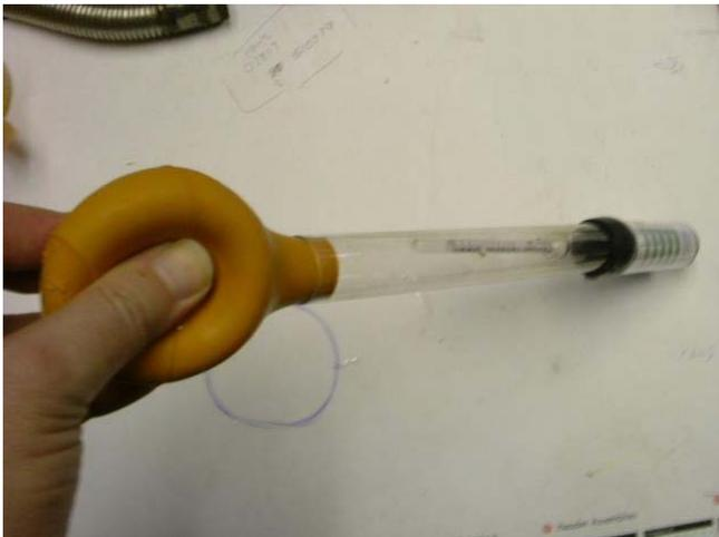
Figure 15.5 - Depress Rubber Bellows
