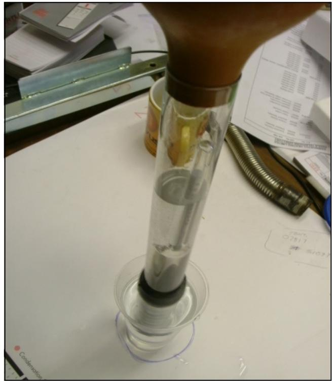
Figure 15.6 - Draw Glycol / Water Solution In Pipette
