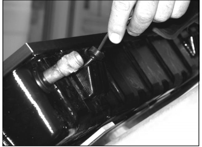
Figure 14.15—Assembly Of Collector Sensor
