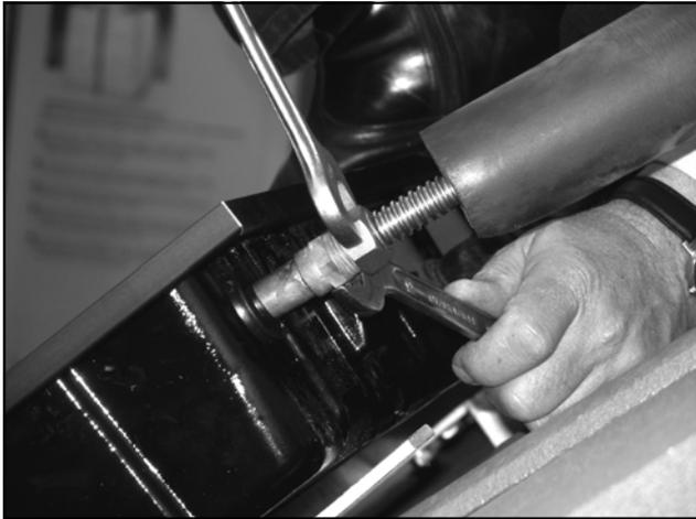
Figure 12.17 - Assembling the hydraulic tube
