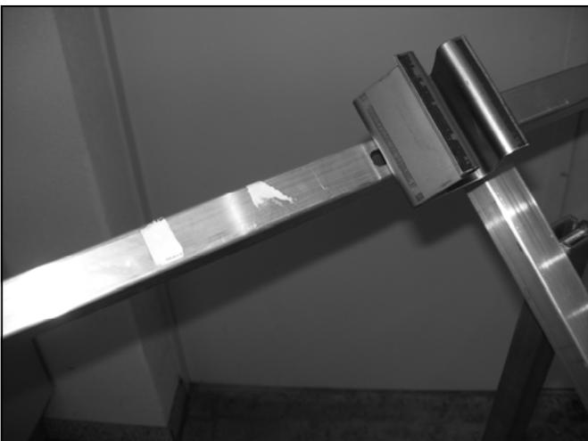
Figure 13.4.16 - Assembly of third triangle with second upper and lower horizontal rail.
