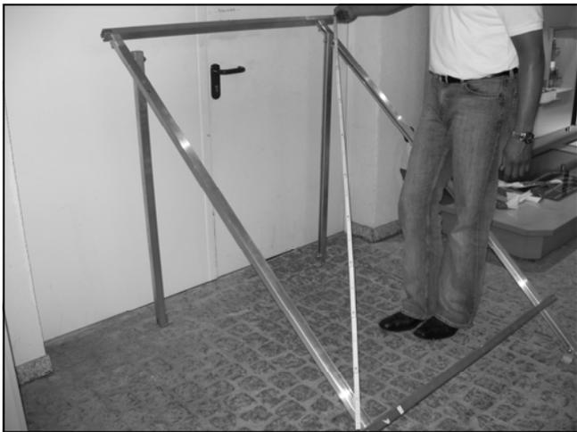
Figure 13.4.11 Checking For A Twisted Frame
