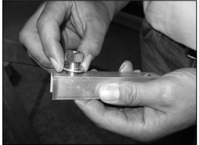
Figure 13.4.13 - Assembly Of Washer And Nut
