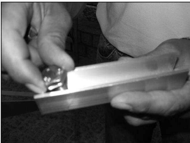
Figure 13.4.12 Assembly Of U-Profile & M12 Screws
