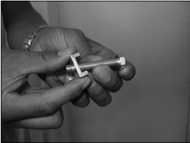
Figure 13.4.1 —Assembly M10 Screw & “U” Washer
