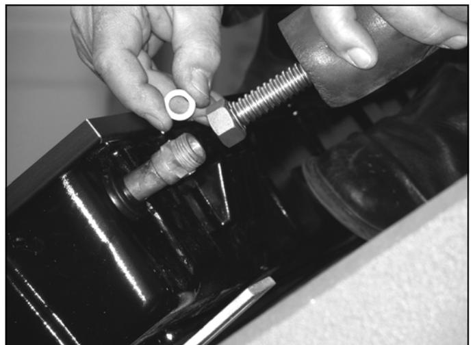
Figure 12.16 Assembling Hydraulic Sealing Ring
