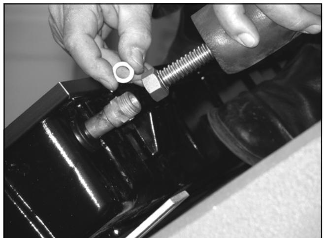
Figure 13.4.21 - Hydraulic Tube Assembly
