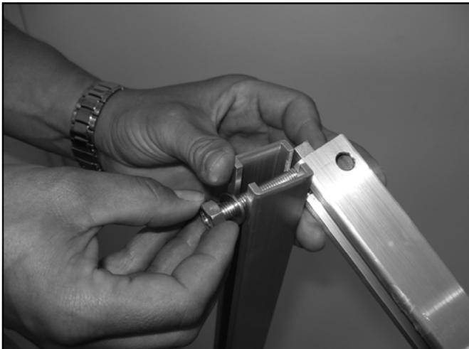
Figure 13.4.2 - Assembly Of 2235mm & 1640mm Long Rails Together.
