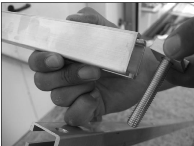
Figure 13.4.7 - Horizontal rail assembly
