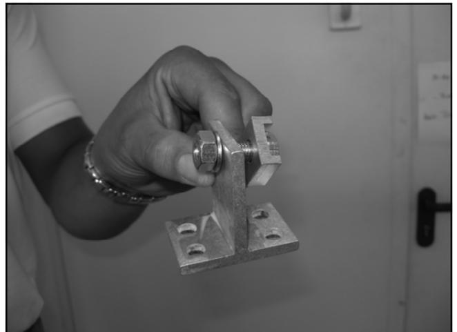
Figure 13.4.4 - Foot Bracket Assembly
