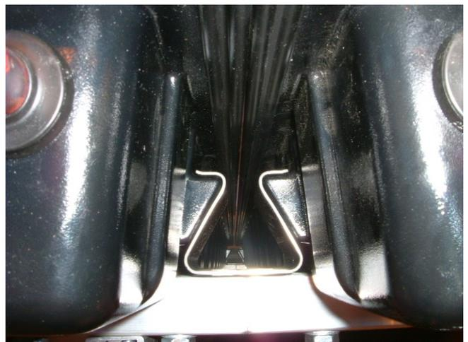
Figure 13.4.17 - Engagement of Double Attachment Clamp With Two Collectors
