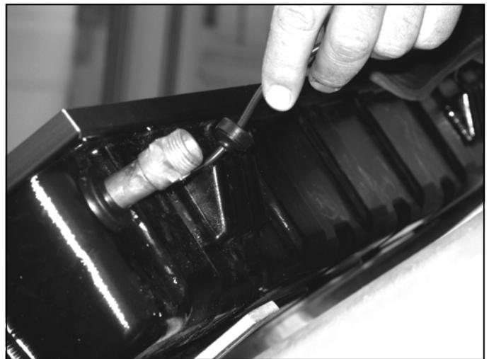
Figure 12.15 Assembly Of Sensor In Collector
