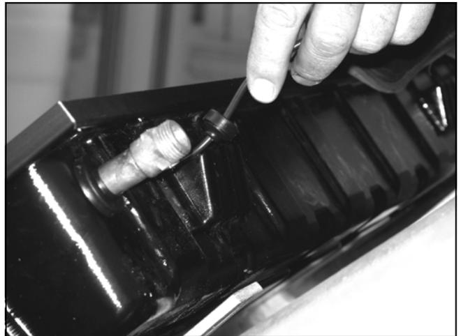
Figure 13.4.20 Assembly Of Collector Sensor
