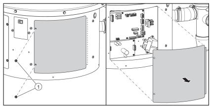
The mains power and optional electrical connections have to be connected to the terminal block of the controller, refer to <u>Structure of the water heater</u> (see 7.1).
