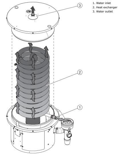
When the temperature is too low, the water heater starts a operating cycle:
