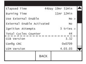
Use the **Appliance Information** submenu to activate or deactivate the external ON mode switch and to set the ignition attempts.
