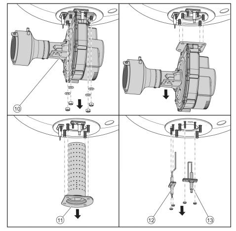
Use compressed air to remove all contamination from the outside to the inside of the burner.
