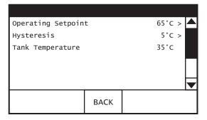
Press on a line with a [>] to set the operating setpoint or to set the hysteresis. Press **[BACK]** to return to the previous screen.
