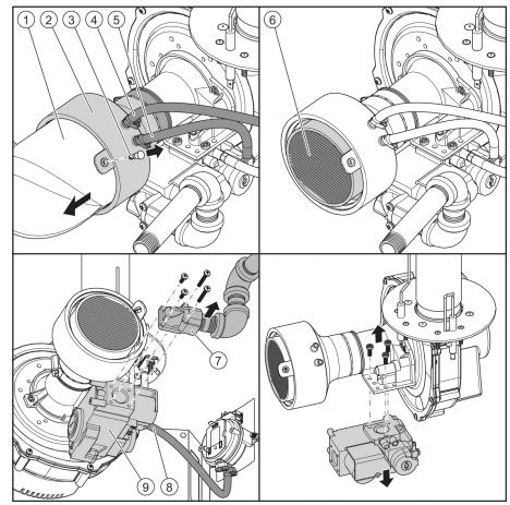
9. Loosen the four nuts to disconnect the fan (10) and the burner (11).
