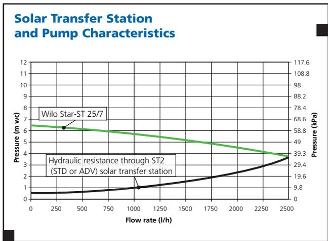
Trigon ST2 (STD or ADV) solar transfer station hydraulic resistance and Wilo Star ST-25/7-3C pump flow characteristics
