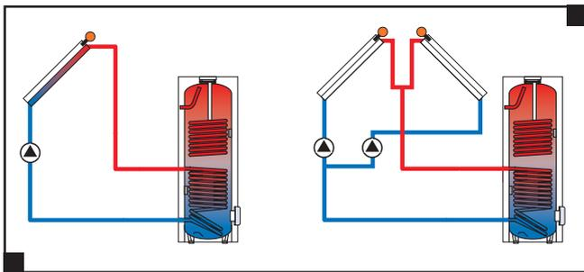
Single collector field and store (left), and dual-collector field and store (right) solar circuits
