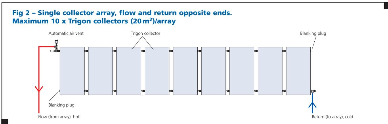
Collector array arrangements complete with hydraulic fittings kit: temperature sensor pocket and sensor, balancing valve for the collector array, automatic air vent (AAV), 3 x Tee connectors (1 capped, 1 with sensor pocket, 1 with AAV and connection nipple), 2 x blanking plugs. Each collector is supplied complete with captive unions and high temperature sealing washers. The appropriate number of flexible connectors are supplied as part of the selected collector mounting kit.
