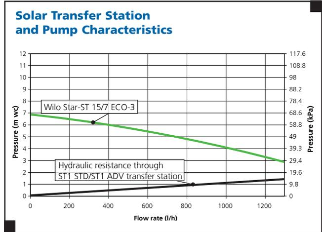
Trigon ST1 (STD or ADV) solar transfer station hydraulic resistance and Wilo Star ST15/7 ECO-3 pump flow characteristics
