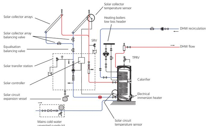
**Scheme B Trigon solar low-volume DHW system, dual collector field**
