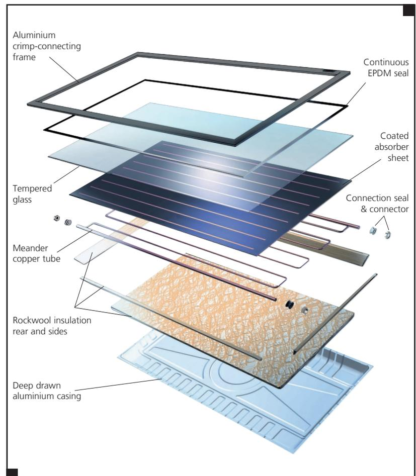
Exploded view of Trigon 2.3H, horizontal, flat plate collector
