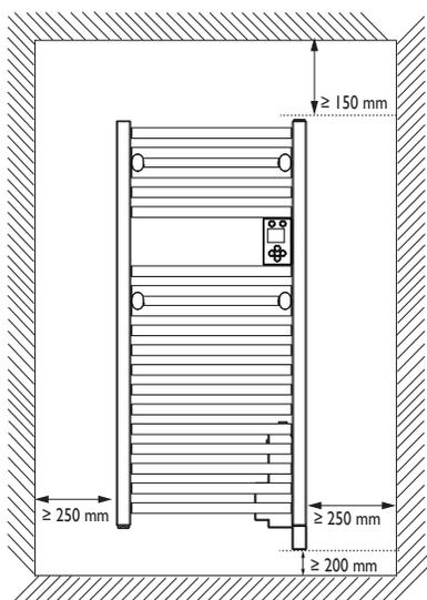
Maintain the minimum distances from furniture when positioning the device. Do not install any shelves above the device.
