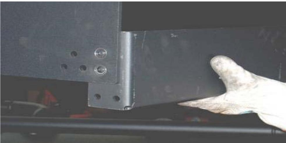
**10.1.4** - Remove from the upper boiler the existing bracing bracket on the lower left and right hand sides. These brackets travel front to rear of the boiler on either side as indicated in Figure 10.1.4.
