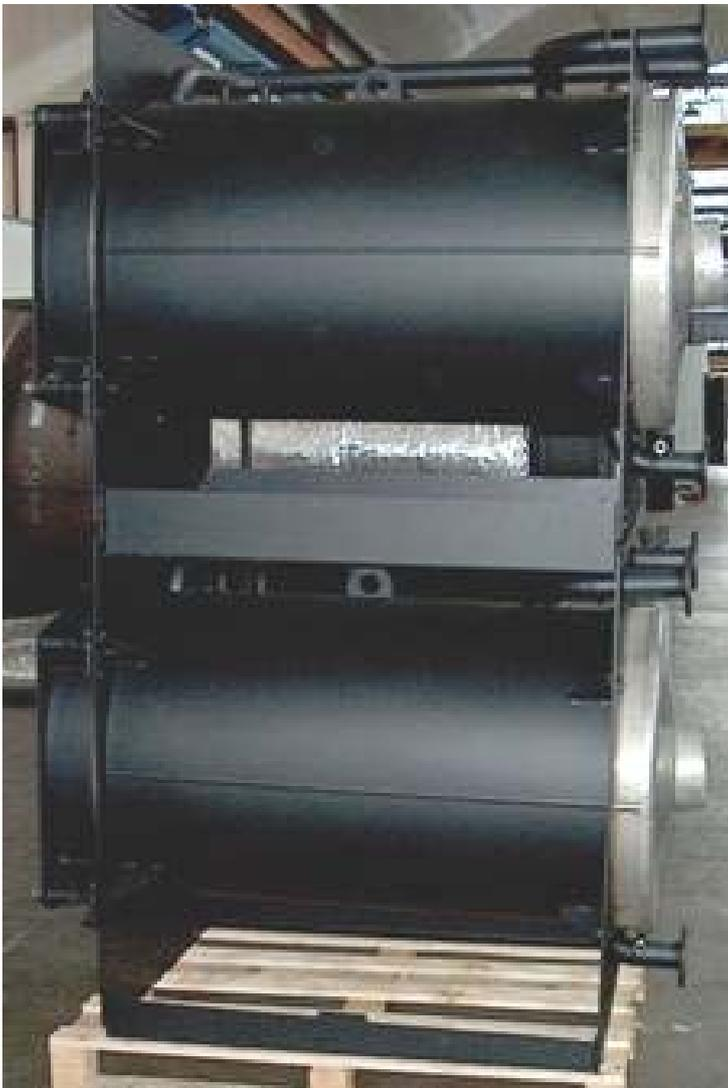
**10.1.10 -** When correctly located the upper and lower boiler front plates should touch. However, the rear plates should have a small gap to ensure the correct slope of the boilers is maintained.
