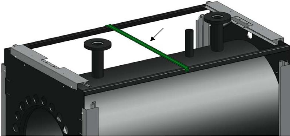
3) Insert the staves, with the previously installed stoppers, between the uprights and the beams, as shown in fig 10.2.3
