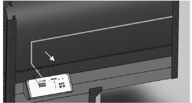
NOTE: if the panel supporting stave is included in the kit (containing the screw holes and the capillary eyelets) it is recommended that you use it to facilitate adjustment; in this case the panel can be installed both on the left-hand and the right-hand side of the wall.
