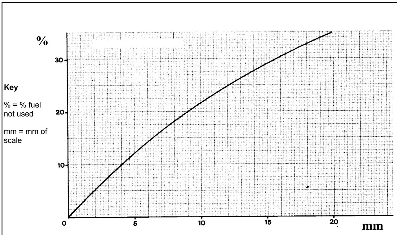
Figure A1.3 - Scale Deposition Chart
