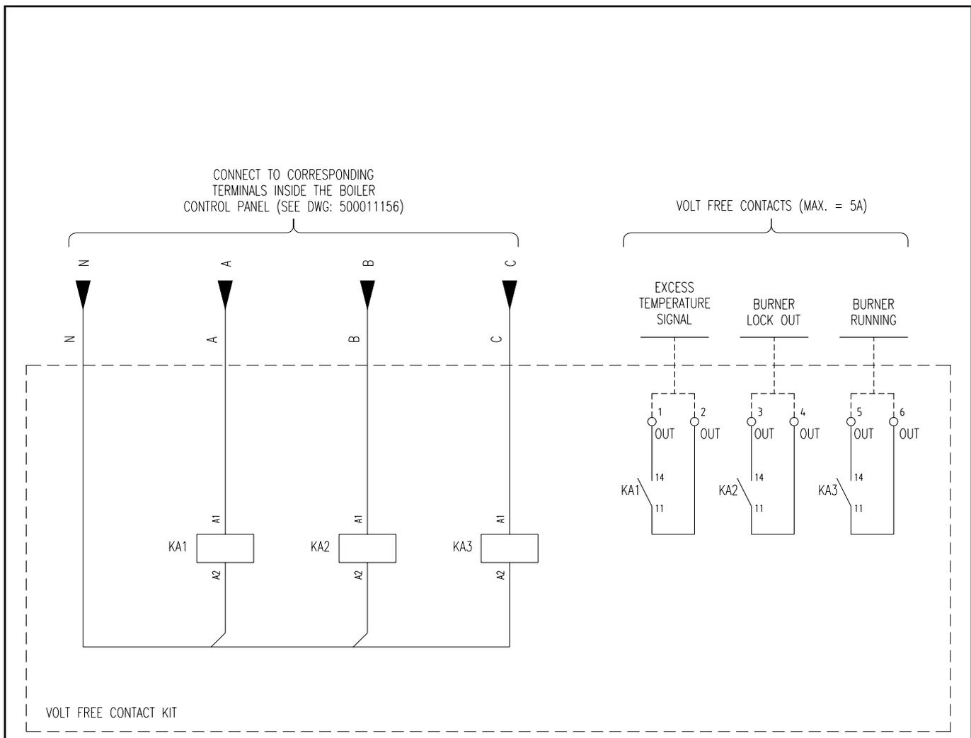
**Figure 9.2 – Volt Free Contact Set and Wiring**
