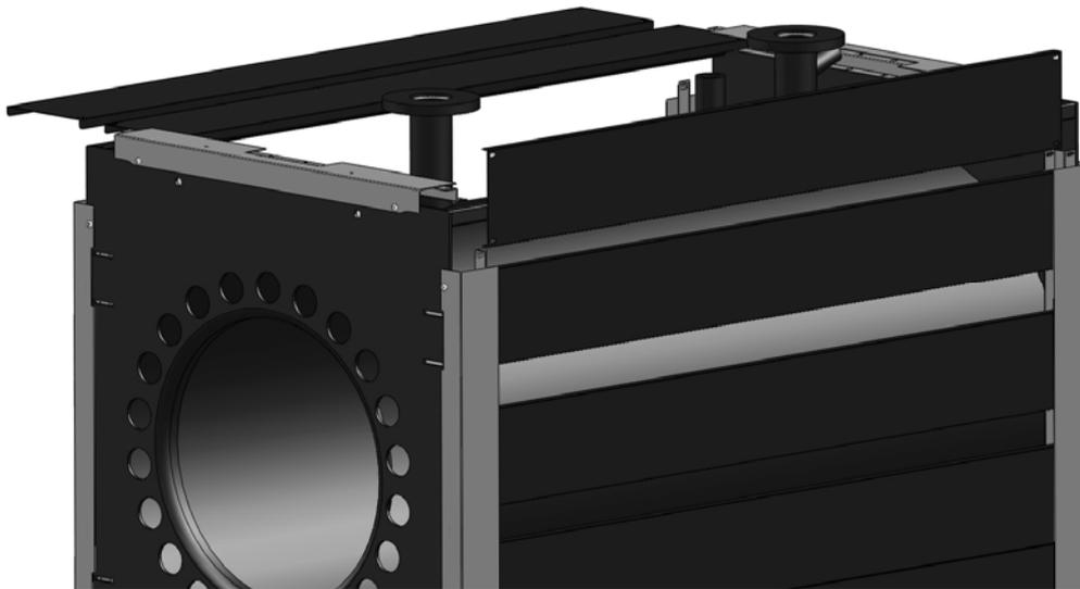
4) After all of the staves have been inserted, install the closing frame using the self-locking screws.
