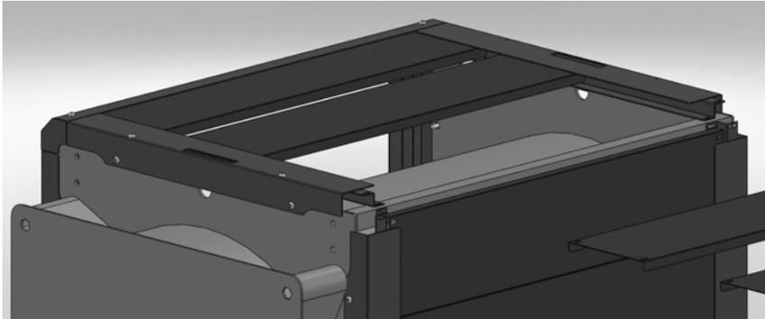
5) After all staves have been fitted, fix the closing frames by self-threading screws.
