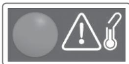
If the overheating LED is lit up, find the cause of overheating and repair if necessary. Once the problem has been solved, it is necessary to manually switch back on the safety thermostat.
