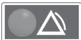
If the external error LED is lit up, refer to the external appliance which is connected to terminals 3, 4 and 5 of the control panel to identify the error, find the cause and eliminate it. It is not necessary to reset the control panel. The display indicating a problem disappears as soon as the error has been removed.
