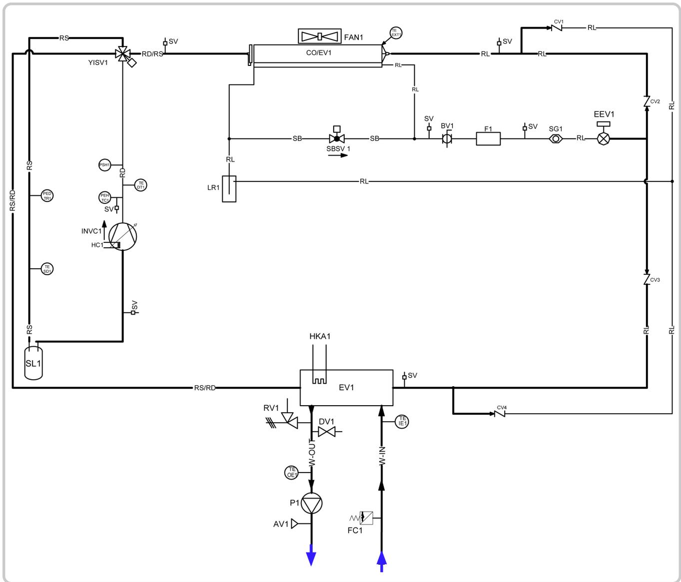
Figure 15 - Operating diagram
