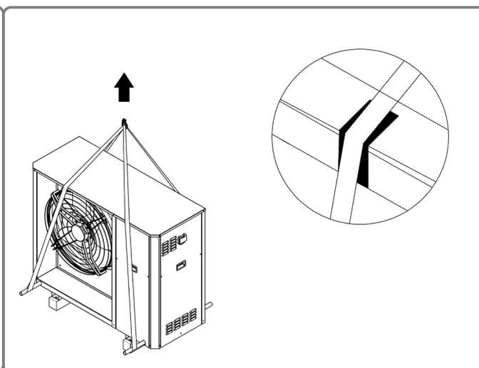
Figure 5 - Lifting with sling system
