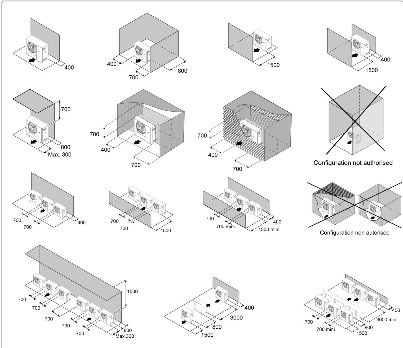
**Figure 8 - Minimum clearances and types of installation**
