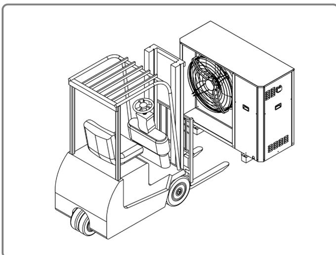
Figure 4 - Lifting with a fork lift truck
