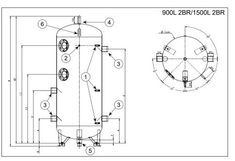
\* Height available to perform the tank drain connection with its isolation valve (not supplied). \*\*No riser provided with the tank
