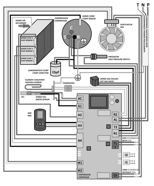
Bobinage compresseur: Compressor winding: RC≈8ohm. CS≈9ohm, SR ≈ 17 ohm, U = 230 V
