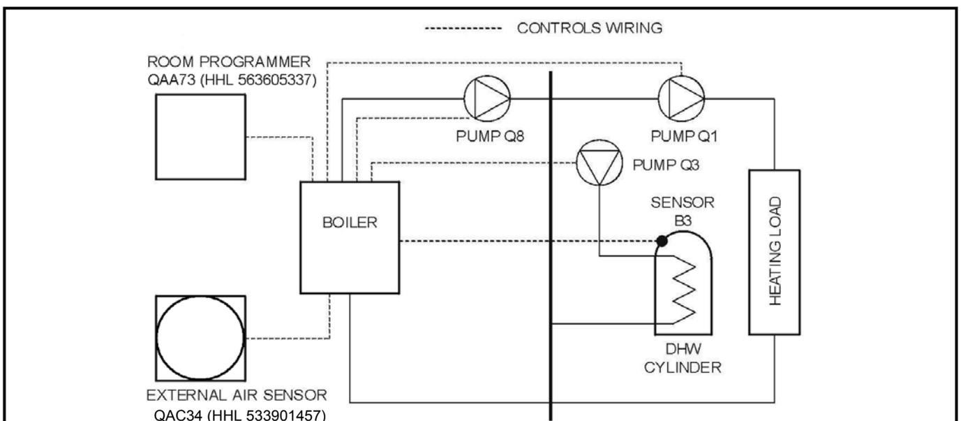
**Figure E 1.3.2 - Schematic for Single Boiler, Primary Circuit System**
