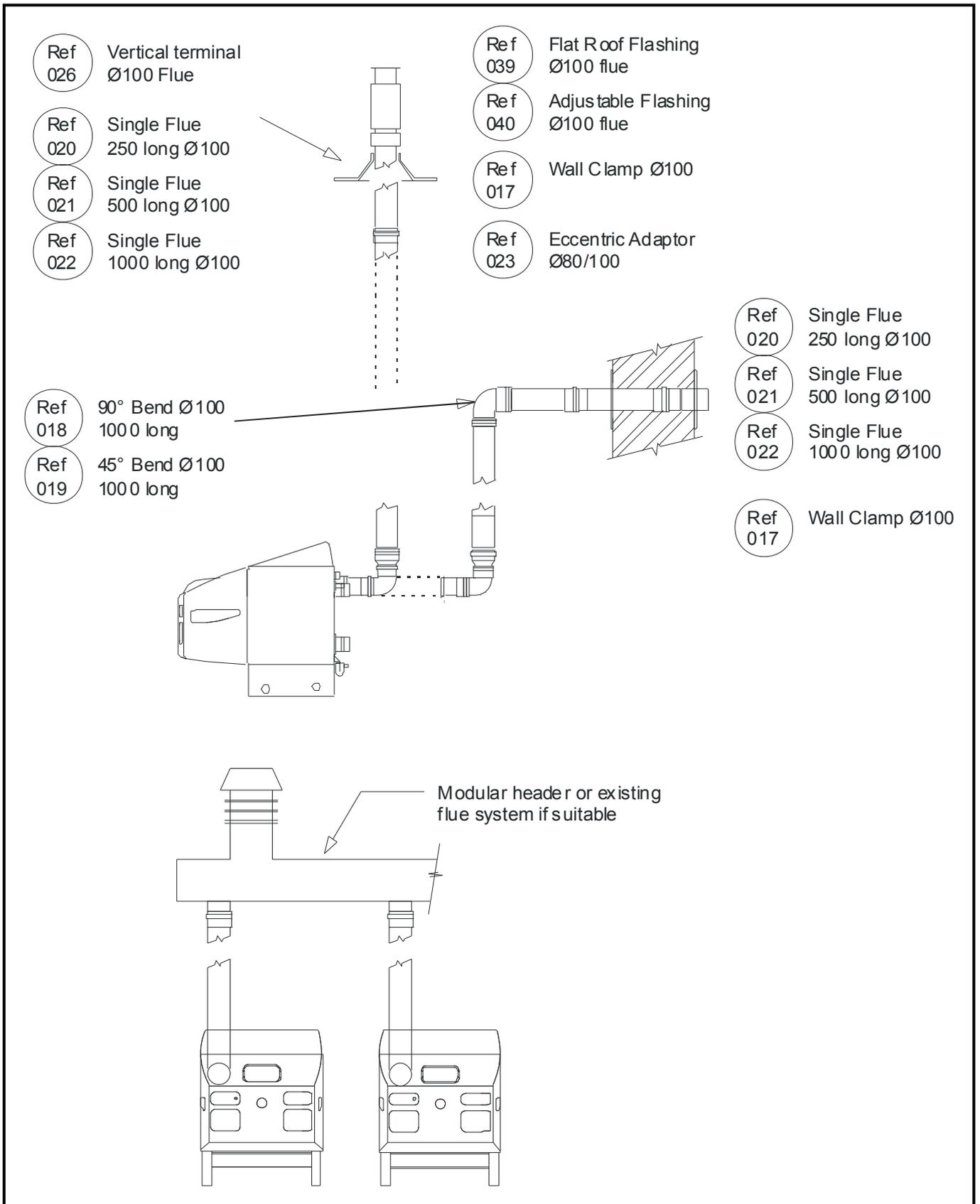
**Figure C1.1.3 - Room Sealed B53 Flue Systems - applies to 100c/110he/120c single boiler installations on-**
