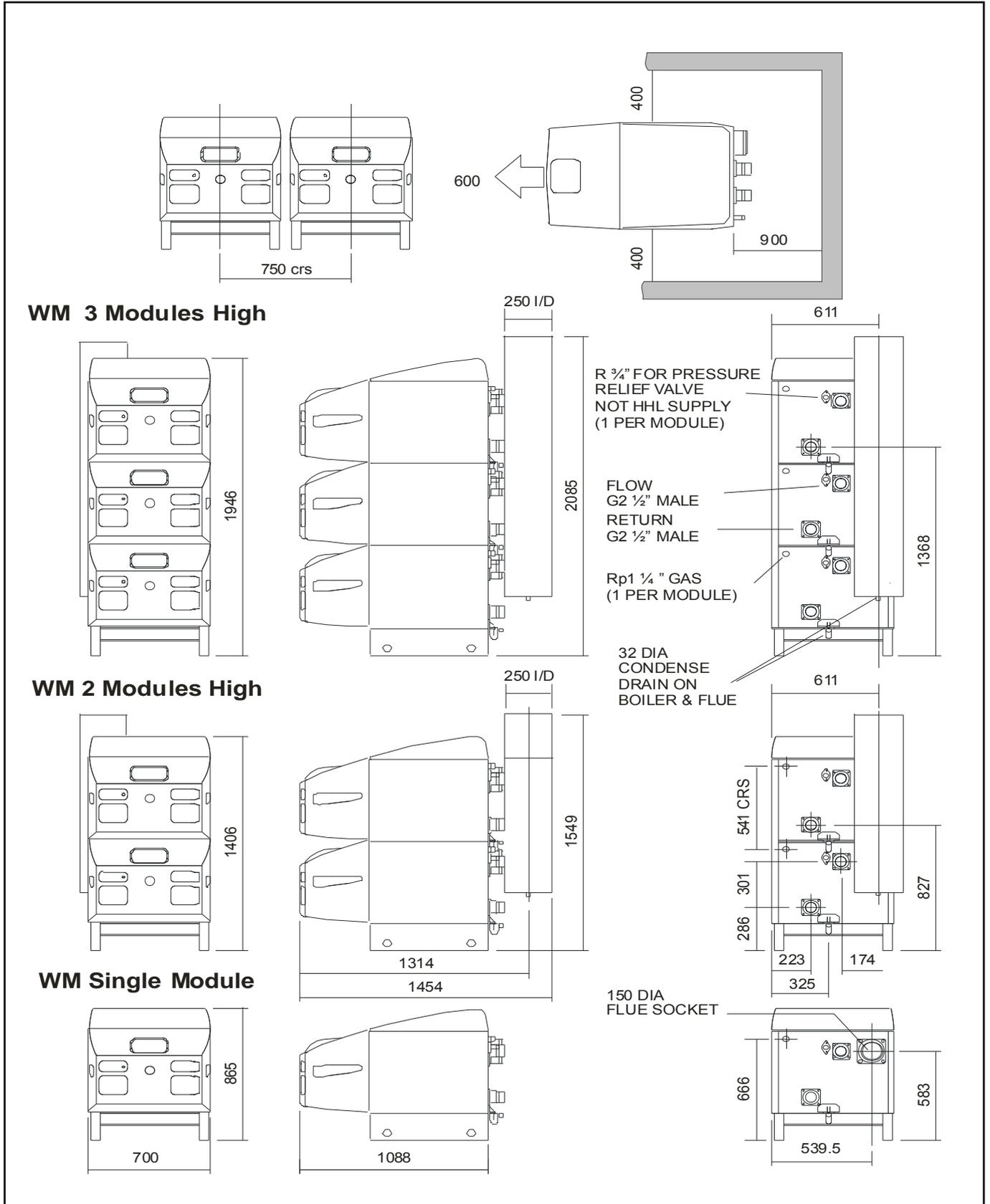
3.2.1 The Hamworthy Heating Ltd water manifold kit is designed to provide a compact solution for connecting the boilers to the gas supply and flow and return water connections. There are two kits specific to individual models. (Refer to the Installer's Guide 500005117 for specific details on the manifold kit, suitable for 100c/110he/120c models)
