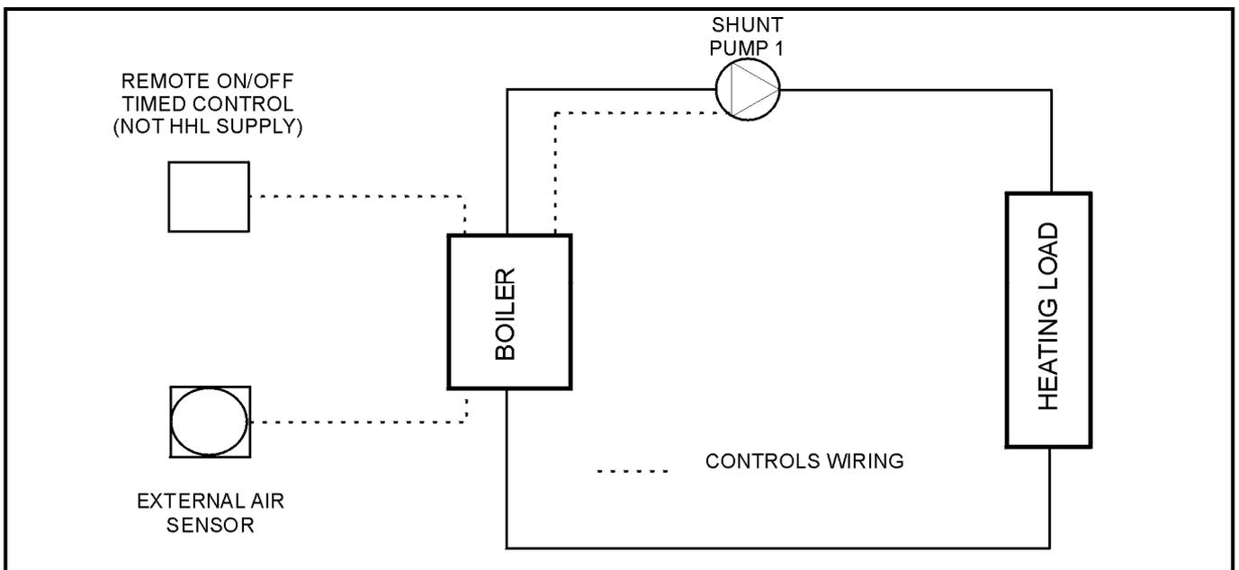
**Figure E 1.3.1 - Schematic for Single Boiler System**
