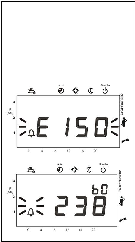
Figure 8.2.4 - Display of lockout code
