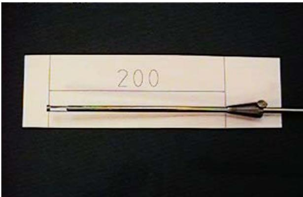
3. Ensure that an insertion distance of 200mm is set on the combustion analyser probe.
