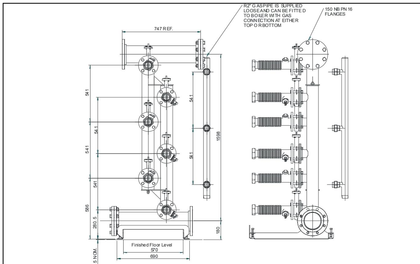
**Figure 3.2.2.2 – Manifold Dimensions for ModuMax 150/450c, 160/480he, 200/600c, 220/660he, 250/750c**
