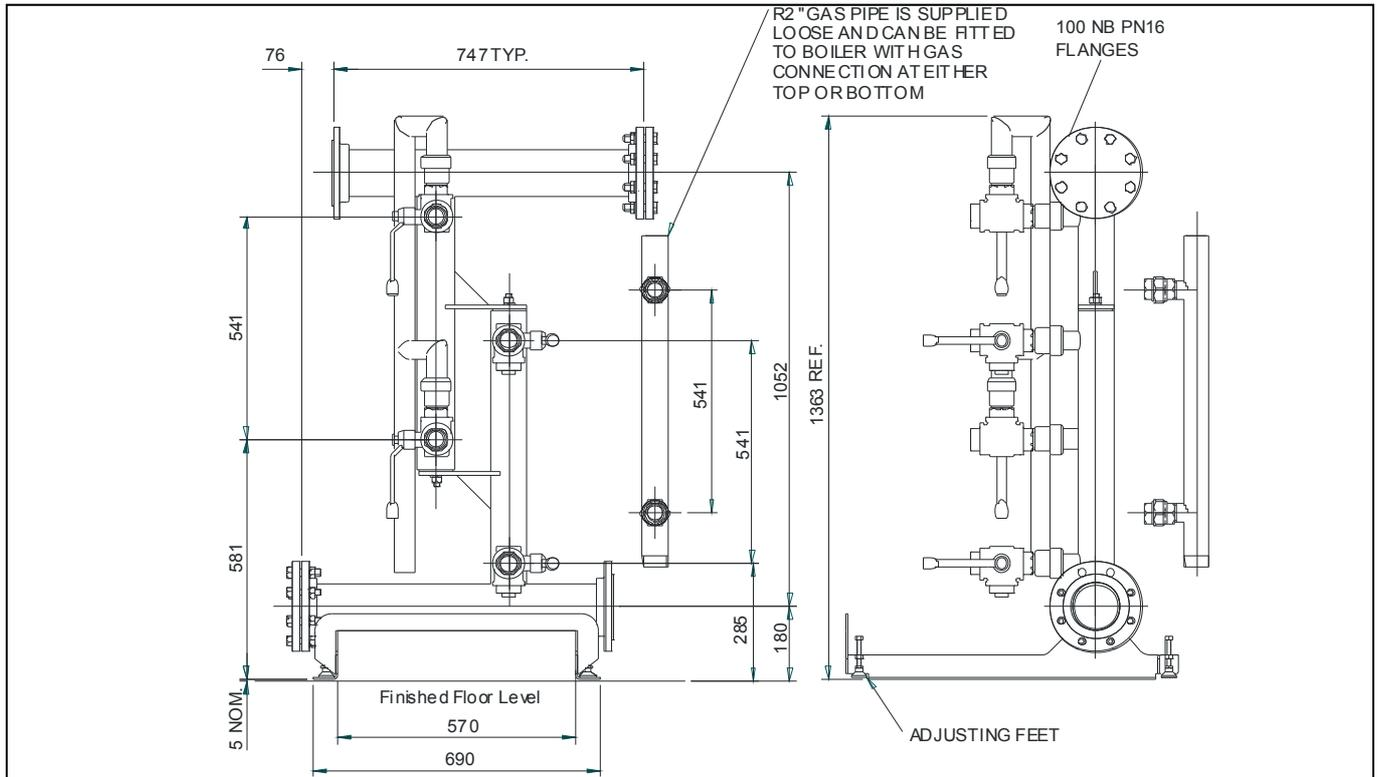
**Figure 3.2.1.1 – Manifold Dimensions for ModuMax 100/200c, 110/220he, 120/240c**
