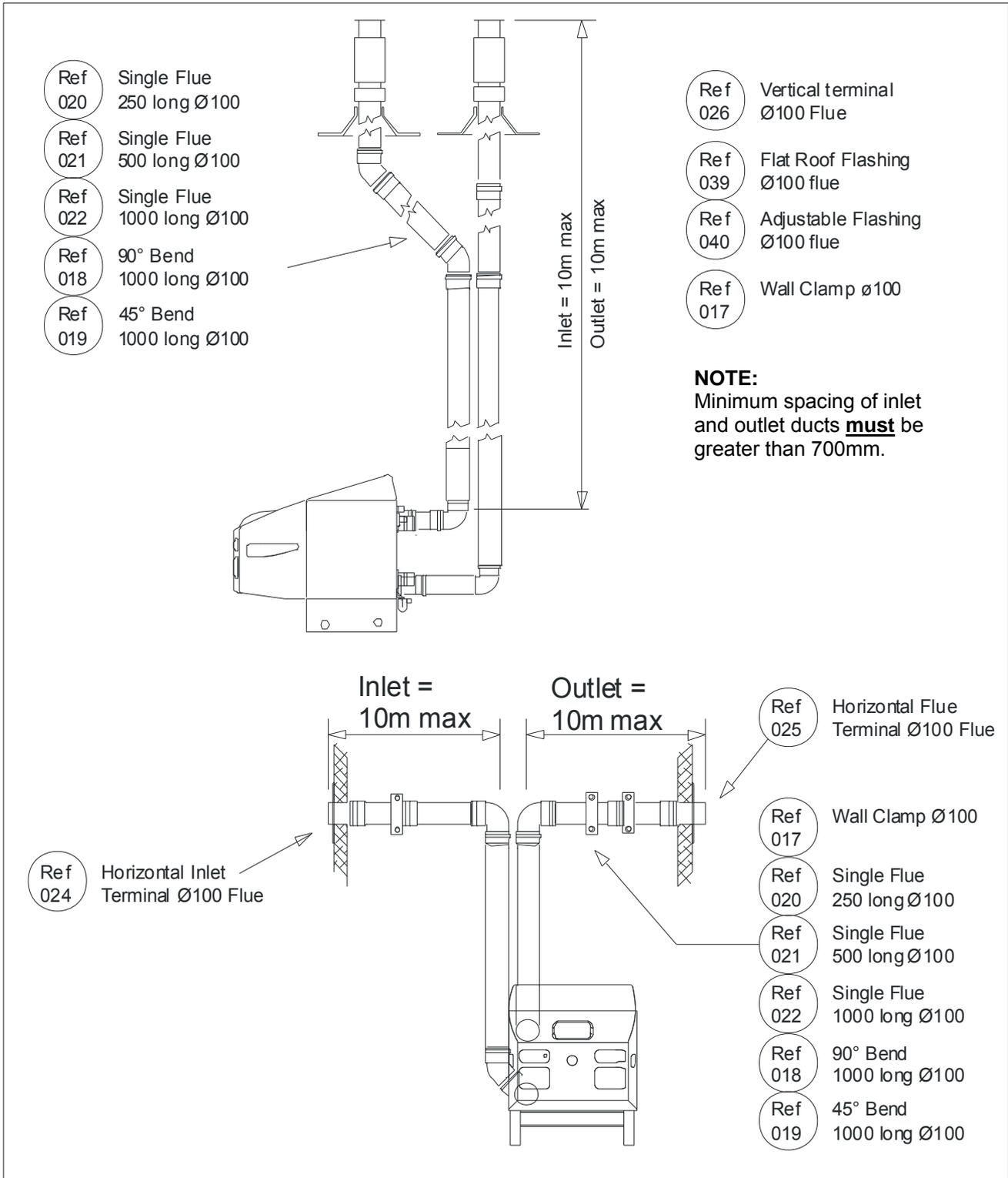
**Connection of 100mm dia. Ducts — Horizontal/Vertical Room Sealed and Open Flue Systems**
