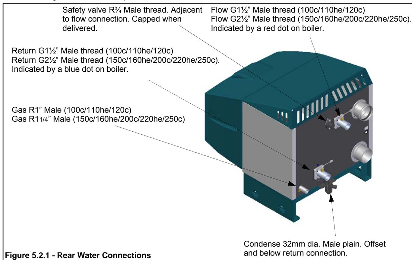
**Figure 5.2.1 - Rear Water Connections**
