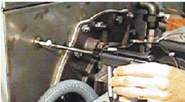
4. Insert probe horizontally into combustion chamber until depth stop is met.
