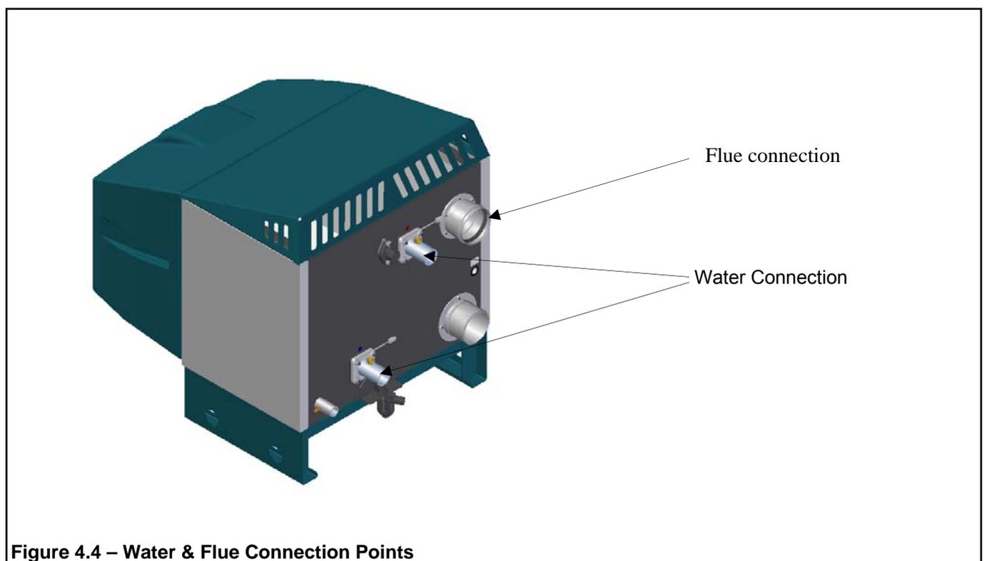
**Figure 4.4 – Water & Flue Connection Points**
