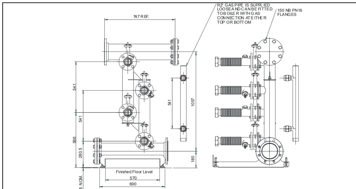
**Figure 3.2.2.1 – Manifold Dimensions for ModuMax 150/300c,160/320he,200/400c, 220/440he, 250/500c**
