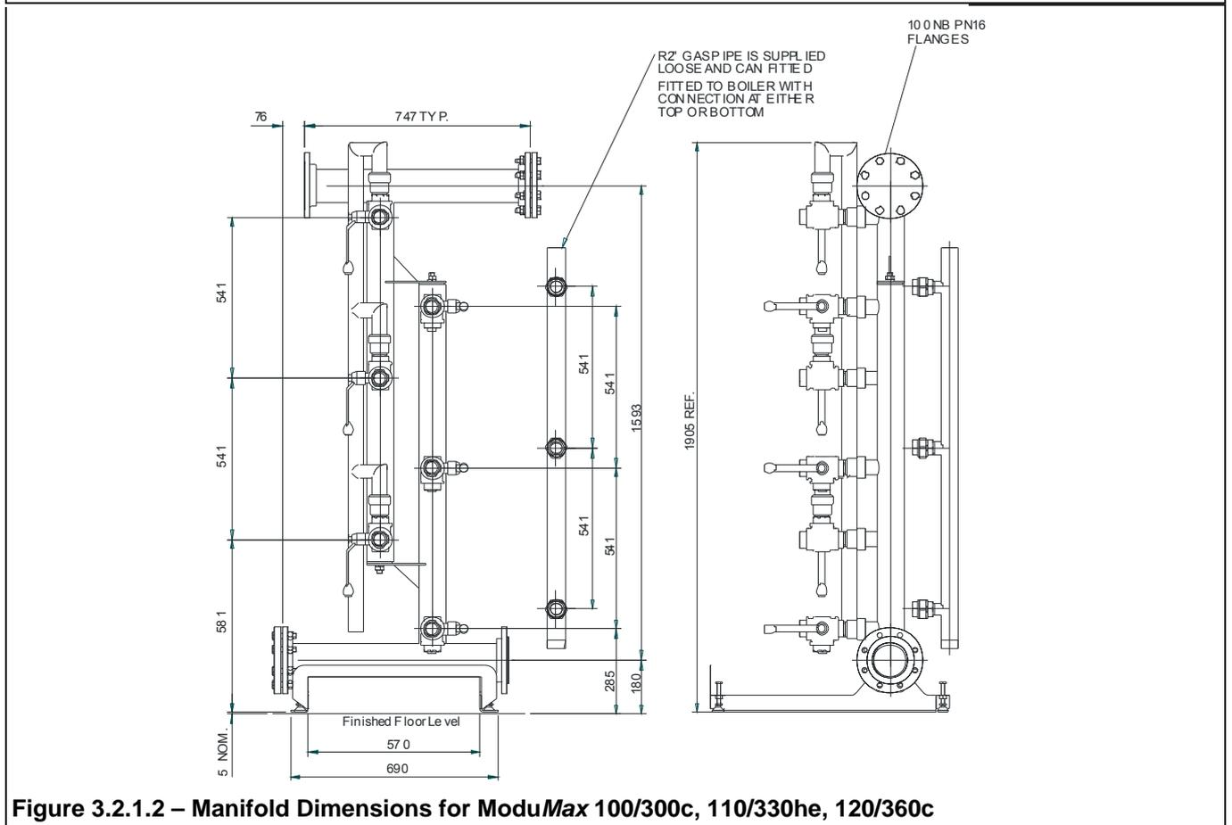
**Figure 3.2.1.2 – Manifold Dimensions for ModuMax 100/300c, 110/330he, 120/360c**
