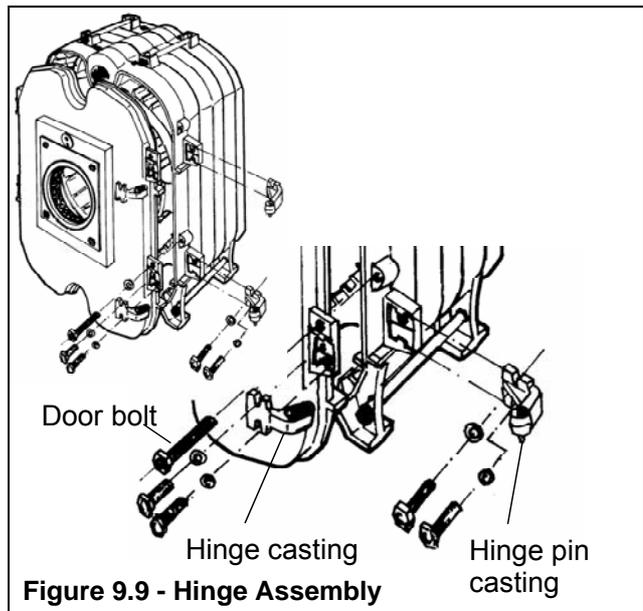
**Figure 9.9 - Hinge Assembly**
