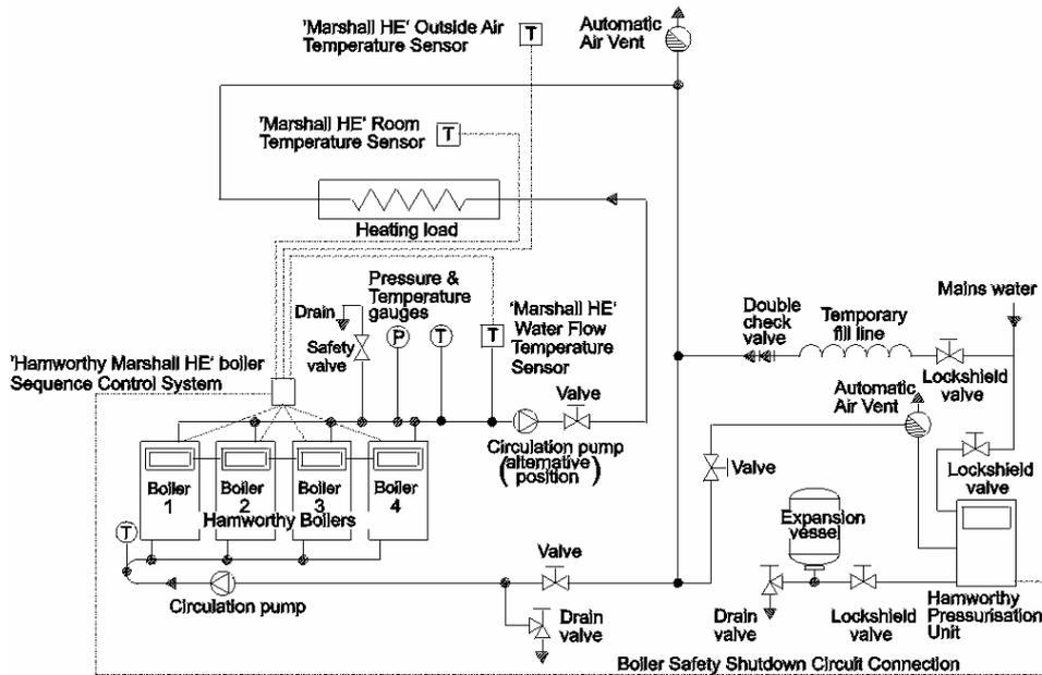
Figure 3.3 - Typical schematic boiler installation layout
