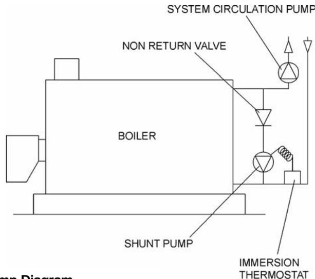
Figure 3.4 - Typical Shunt Pump Diagram
