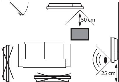
To optimize the absence detection of your device, avoid installing it in a closed corner or behind a piece of furniture.
