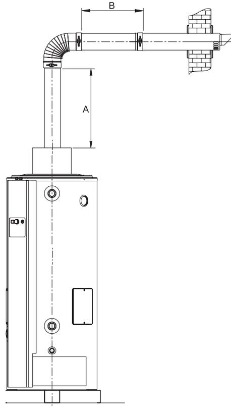
Figure 3.5 Wall flue terminal
