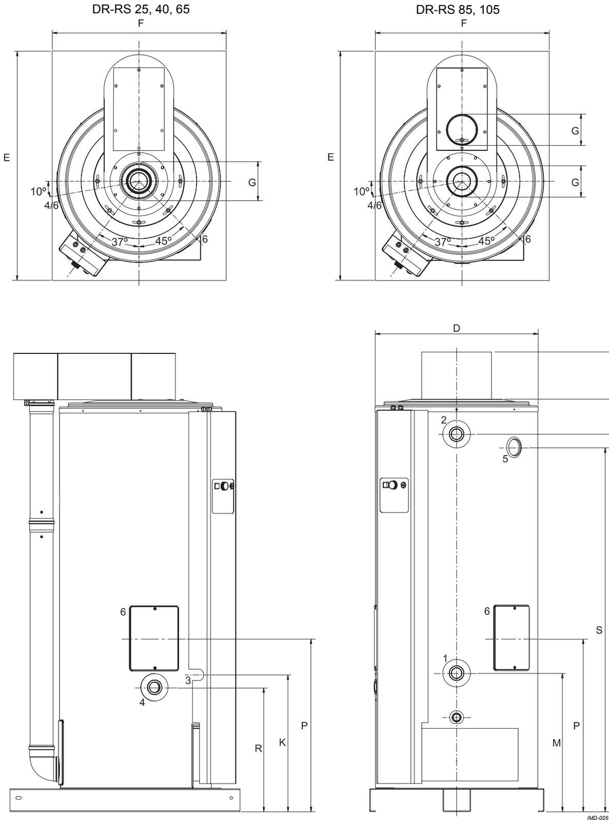
Figure 3.2 Plan and elevation of the water heater
