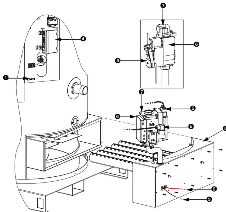
Figure 3.12 Disassembled gas control
