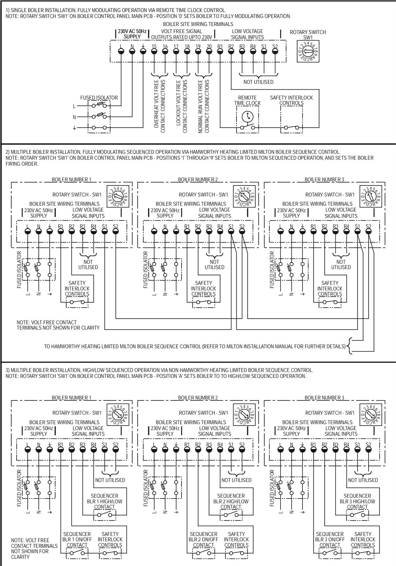
**Figure 8.12 Site Wiring Diagram (Page 2 of 2)**
