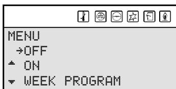
5. Press once on the blue arrow (↓) to position the cursor beside **ON**, then press **ENTER**. The display shown in the figure will appear.
