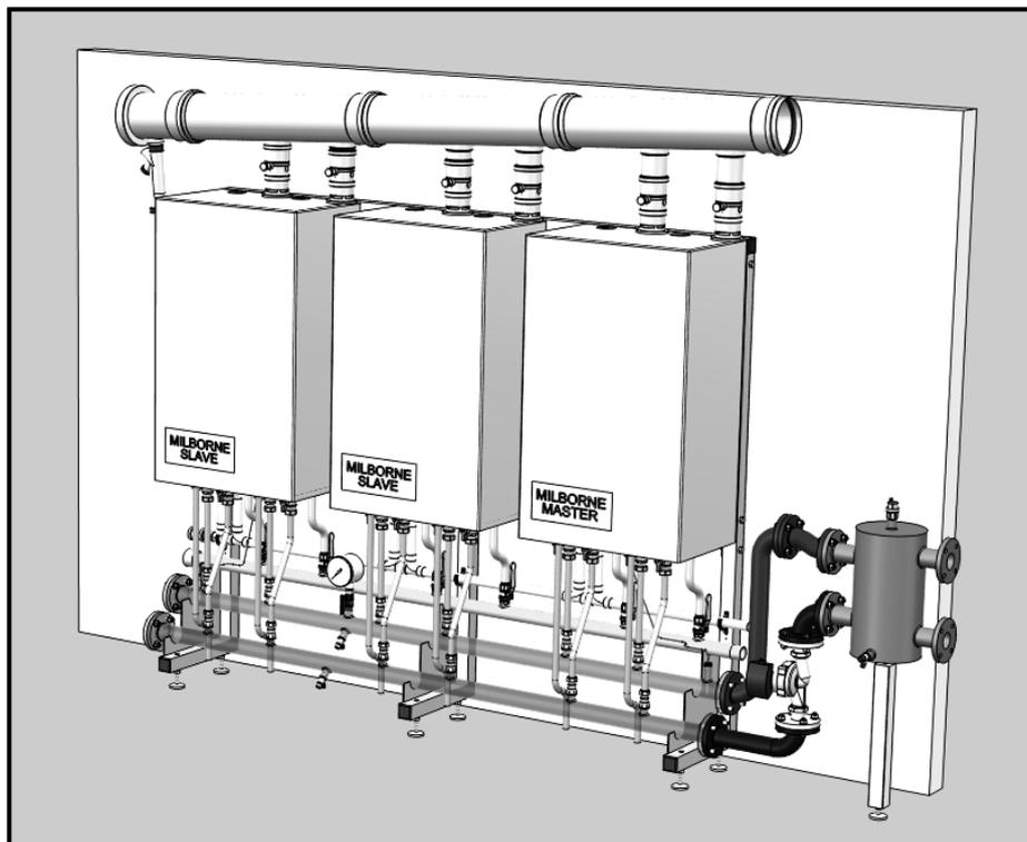
Figure 2.5 - Three boiler arrangement showing frame, flue header, water pipework and primary circuit pump kit
