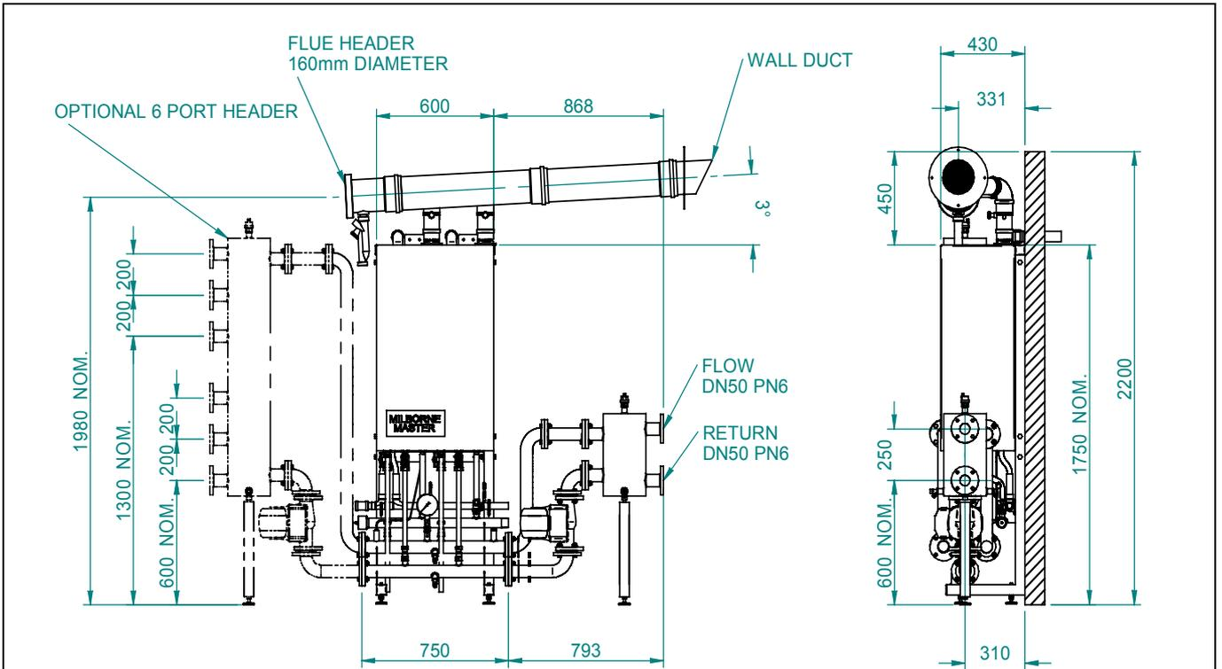
Figure 3.2.1 – Single boiler installation dimensions - room sealed
