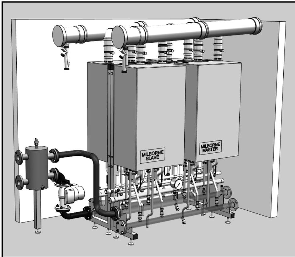
**Figure 2.6 - Two boiler back to back arrangement showing frame, flue headers, water pipework and primary circuit pump kit**
