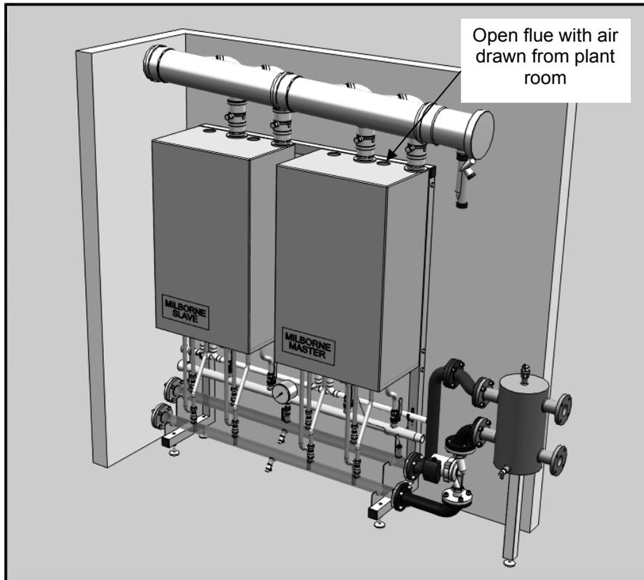
Figure 2.4 - Two boiler arrangement showing frame, flue header, water pipework and primary circuit pump kit
