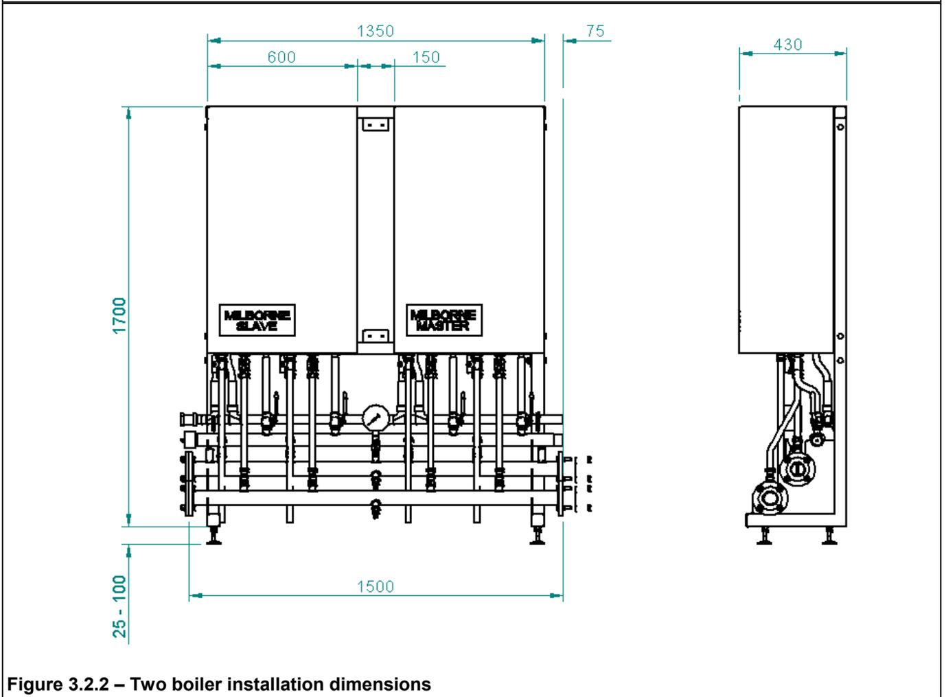
Figure 3.2.2 – Two boiler installation dimensions
