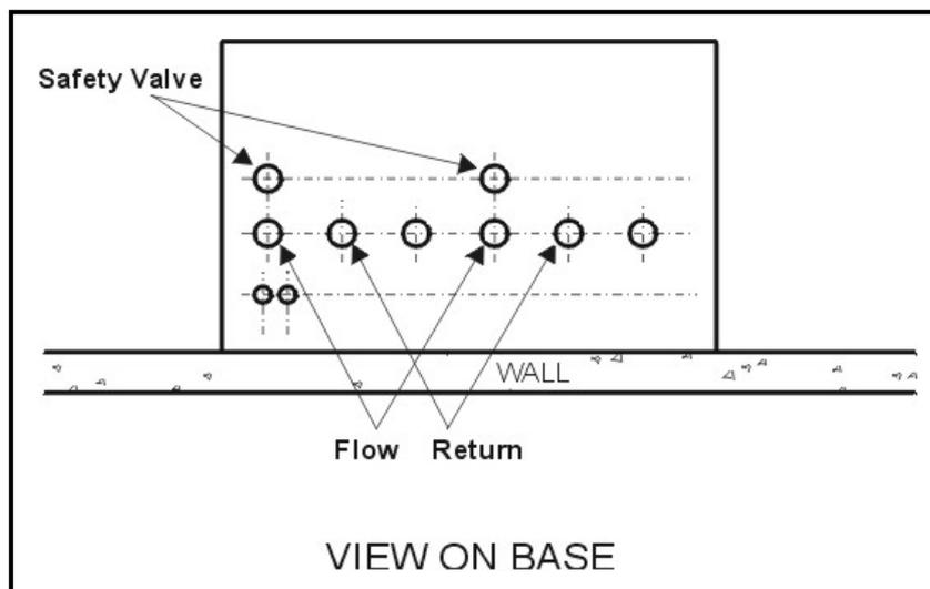
Figure 4.4 - Water Connection Point
