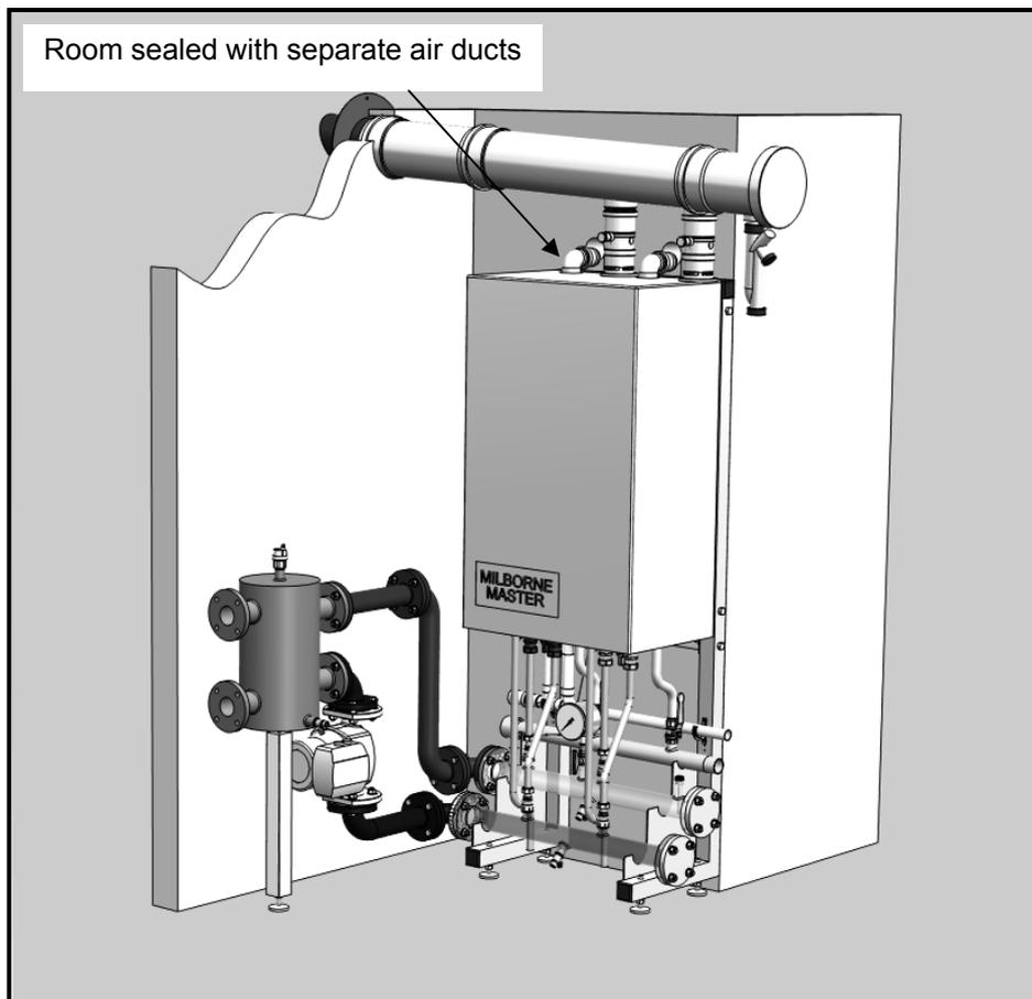
**Figure 2.3 - Single boiler arrangement showing frame, flue header, water pipework and primary circuit pump kit**
