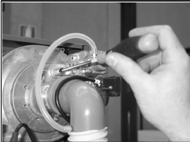
**Fig 7.4.8 - Throttle Adjustment**
