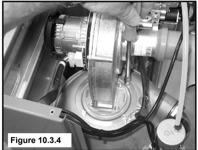
Unscrew the 4 nuts locking the flange onto the burner head and remove the fan as shown in figure 10.3.4
