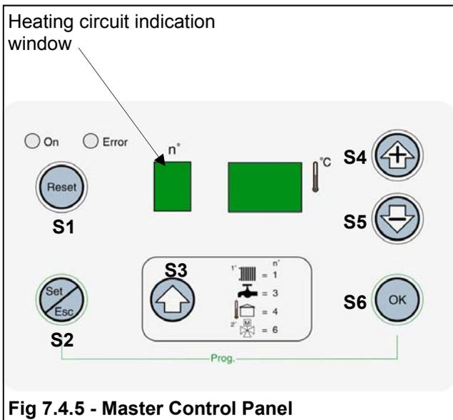
**Fig 7.4.5 - Master Control Panel**
