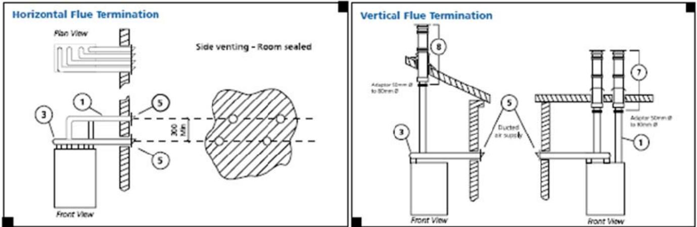
**Figure 5.2.2.4 - Single Milborne - Room Sealed Flue Installation**
