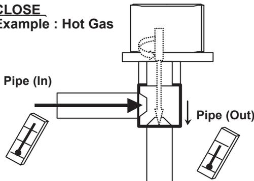
If it is open, it has no temp. difference between Inlet and Outlet.
