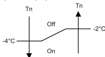
When the jumper wire (JM2) is disconnected:
