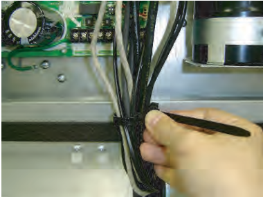
Loose or remove the cable ties. (3 places)
