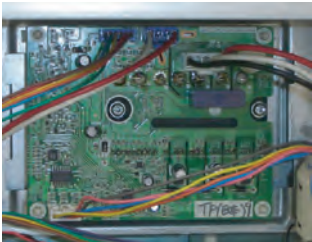
Remove the connectors.
