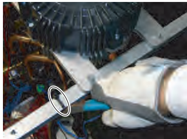
Cut the cable tie.
