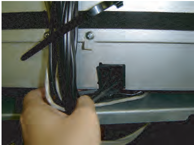
Remove the wires from edging saddle. (3 places)
