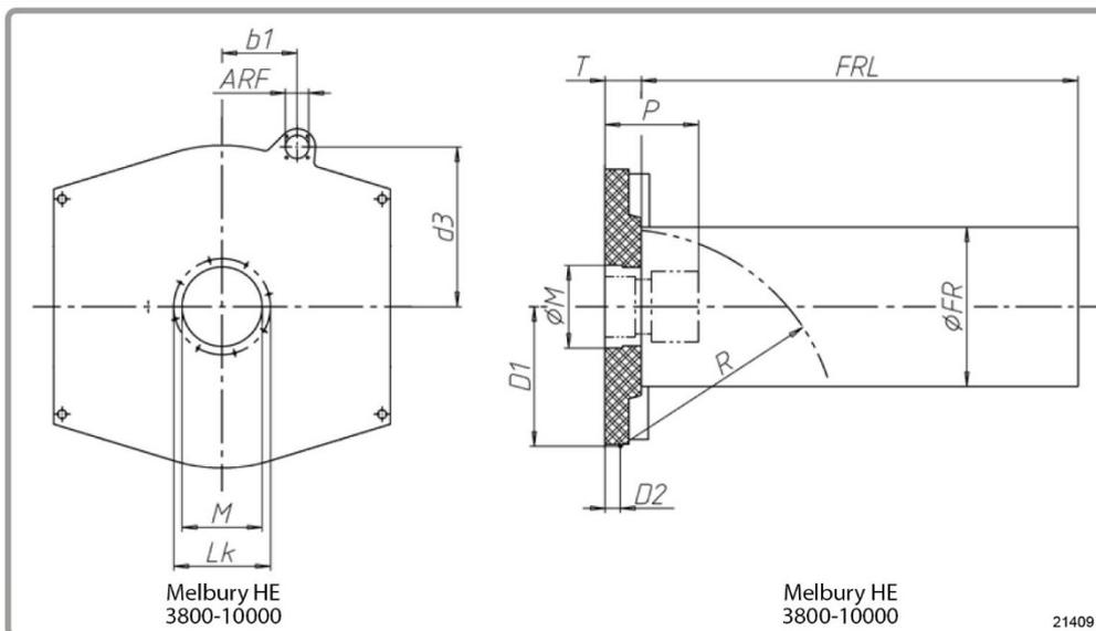
figure 12 - Burner mating dimensions for Melbury BE
