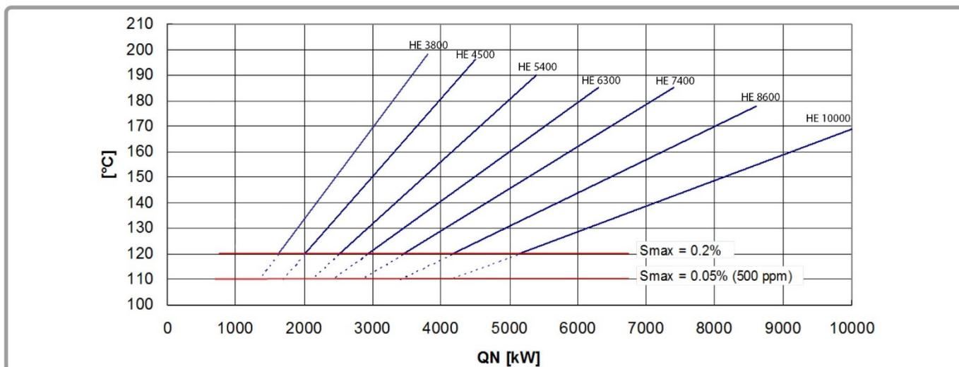
figure 5 - Flue gas temperature diagram Melbury HE, fuel oil with clean boiler
