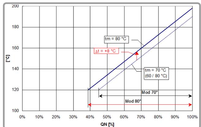
figure 7 - Flue gas temperature – Boiler power diagram (example for two average boiler water temperatures)
