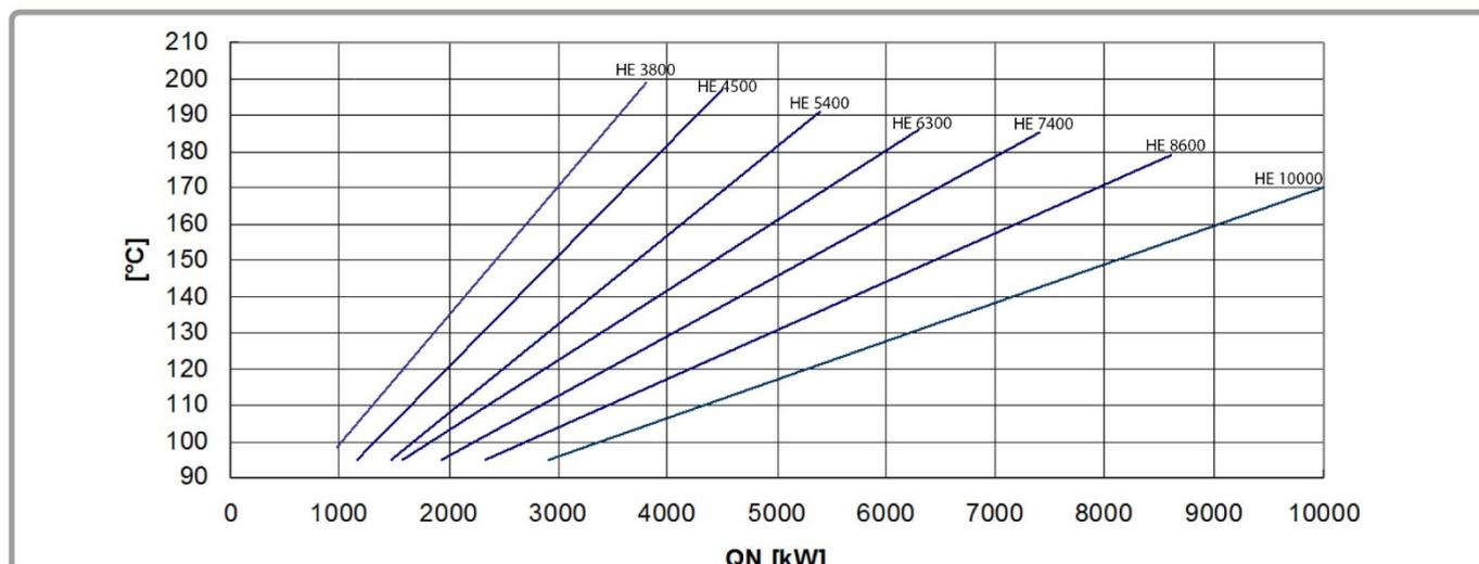
figure 6 - Flue gas temperature diagram Melbury HE, natural gas with clean boiler
