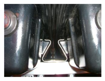
Figure 13.4.17 - Engagement of Double Attachment Clamp With Two Collectors
