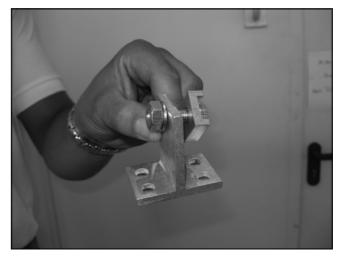
Figure 13.4.4 - Foot Bracket Assembly
