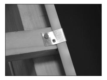
Figure 14.6 – Plate Holder Assembly
