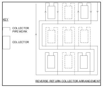
Figure 3.16 - Reverse Return Header Arrangement
