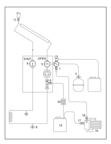
Figure 15.9 - Hydraulic Circuit For Priming Filling Pump
