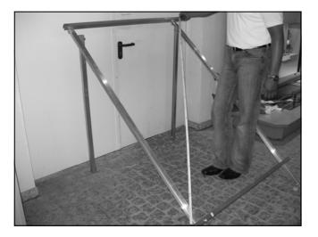
Figure 13.4.11 Checking For A Twisted Frame
