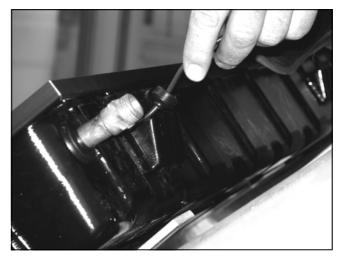
Figure 13.4.20 Assembly Of Collector Sensor
