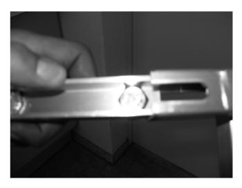
Figure 13.4.14 - U-Profile Rail Assembly To Horizontal Rails
