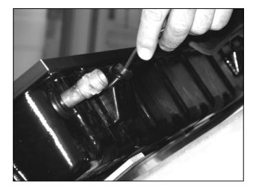
Figure 12.15 Assembly Of Sensor In Collector
