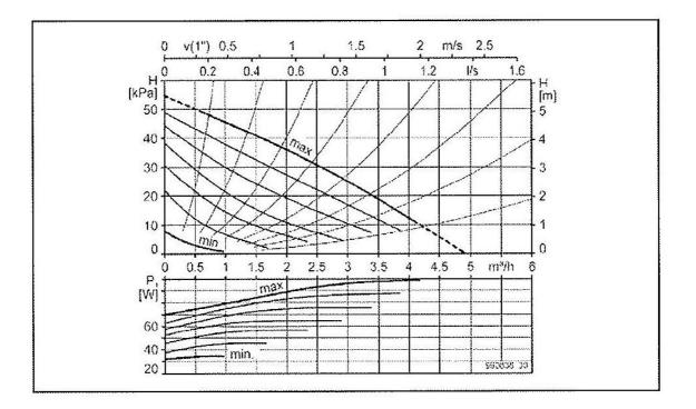
Figure A1 - Pump Characteristics Curve
