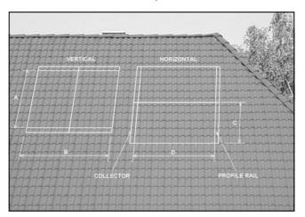
Figure 12.3 - Collector Position On Roof
