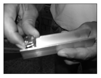
Figure 13.4.12 Assembly Of U-Profile & M12 Screws
