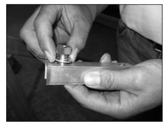
Figure 13.4.13 - Assembly Of Washer And Nut
