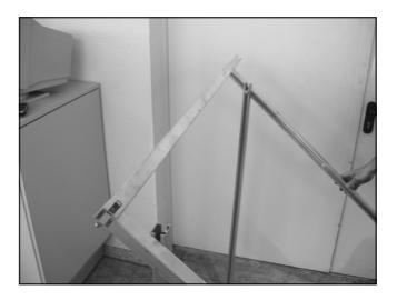
Figure 13.4.9 - Assembly Of Upper Horizontal Rail
