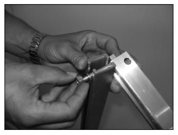
Figure 13.4.2 - Assembly Of 2235mm & 1640mm Long Rails Together.
