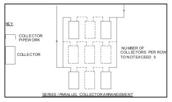
Figure 3.15 - Collector Array Balancing
