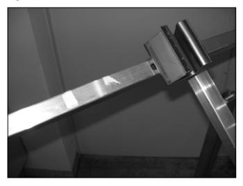
Figure 13.4.16 - Assembly of third triangle with second upper and lower horizontal rail.
