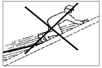
Figure 12.5 - For safety do not step on attachment rail
