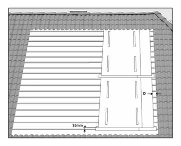
Figure 14.5 - Assembly Of Collector Plates
