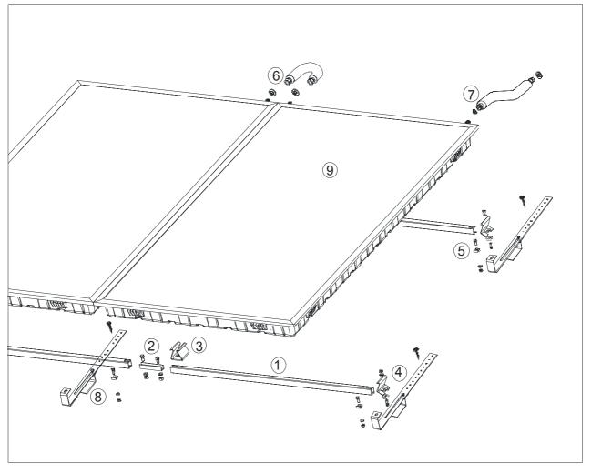
Figure 12.2 - Exploded View Of Vertical On-Roof Collector Arrangement
