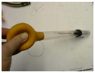
Figure 15.5 - Depress Rubber Bellows
