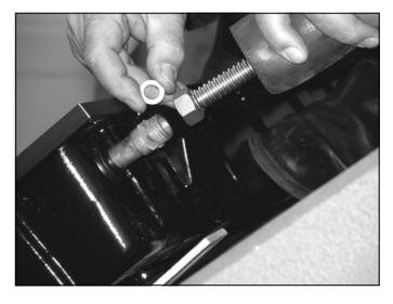
Figure 12.16 Assembling Hydraulic Sealing Ring
