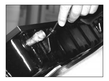
Figure 14.15—Assembly Of Collector Sensor
