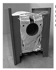
Hook the RH and LH side covers over the spacers and tie rods and secure using the nuts and bolts.
