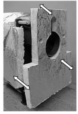
Fit the rear insulation jacket over the flue outlet. Secure the top and side edges of the rear jacket to the wrap using duct tape
