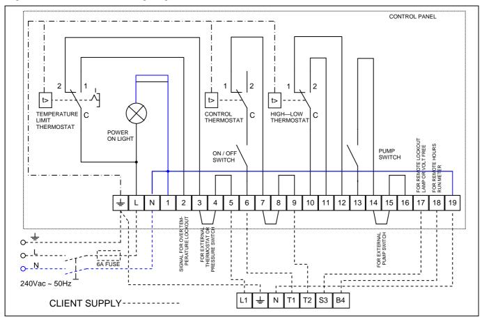
Fig. 6. Boiler Control Panel Wiring Diagram For 7 Pin Burner Plug
