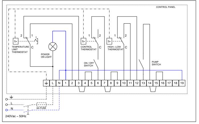
Fig. 2. Boiler Control Panel Wiring Diagram
