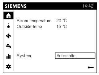
The start page for the QAA74 room unit displays the most important information on the room and plant/zone switch.
