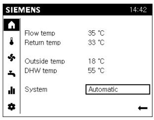
The start page for the AVS74 operator unit displays the most important information on the energy producer and plant/zone switch.
