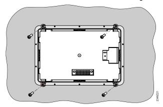
Attach the unit to the source housing using 4 screws.
