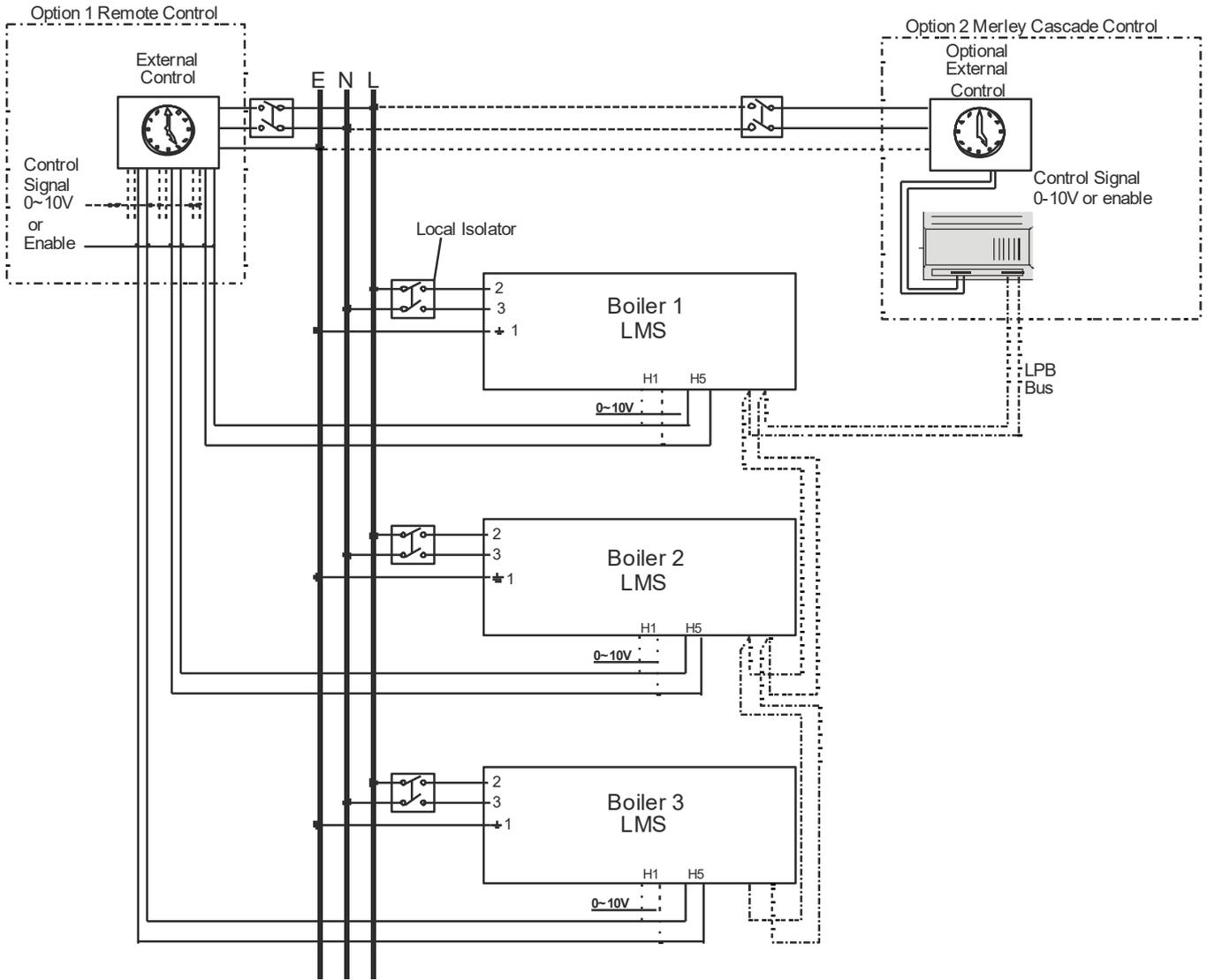
**Note:-** each module requires independent isolation of electrical supply and control signals. Signal cables must not be run in the same conduit as mains voltage cables
