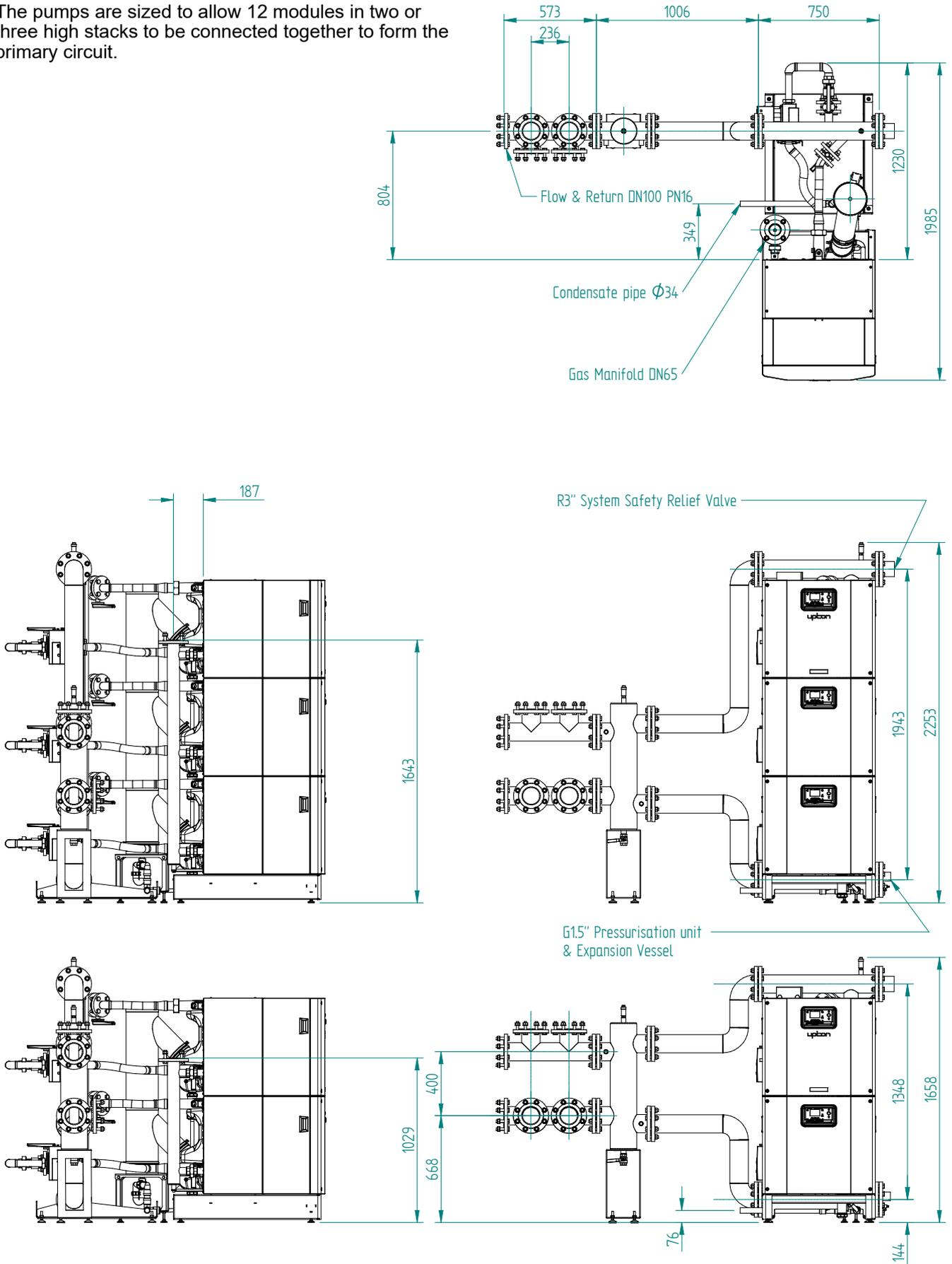
Figure 3.2.2 – UF100 & UF150 2MW Primary circuit and Gas manifold pipe kit
