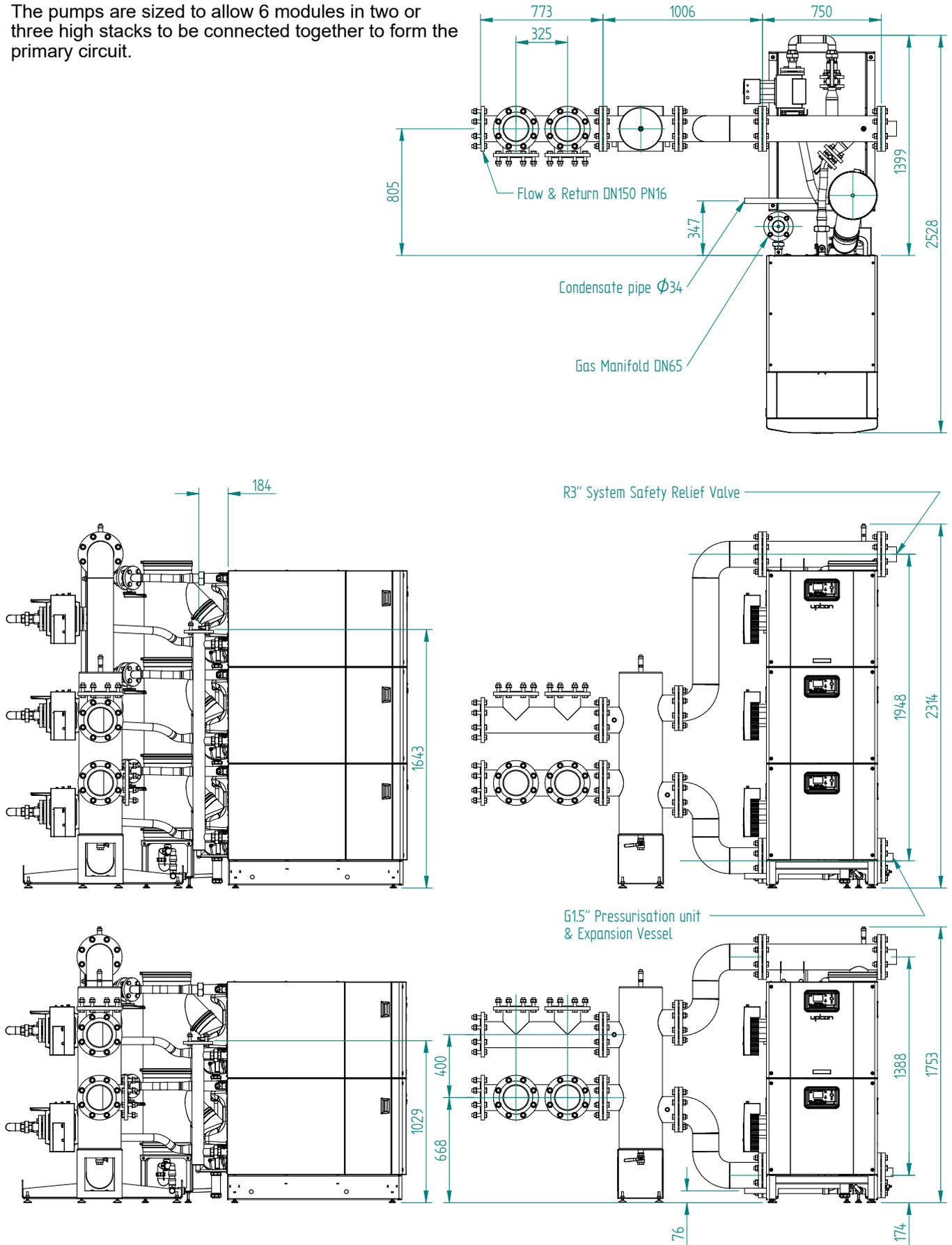
Figure 3.2.4 – UF300 & UF350 2MW Primary circuit and Gas manifold pipe kit
