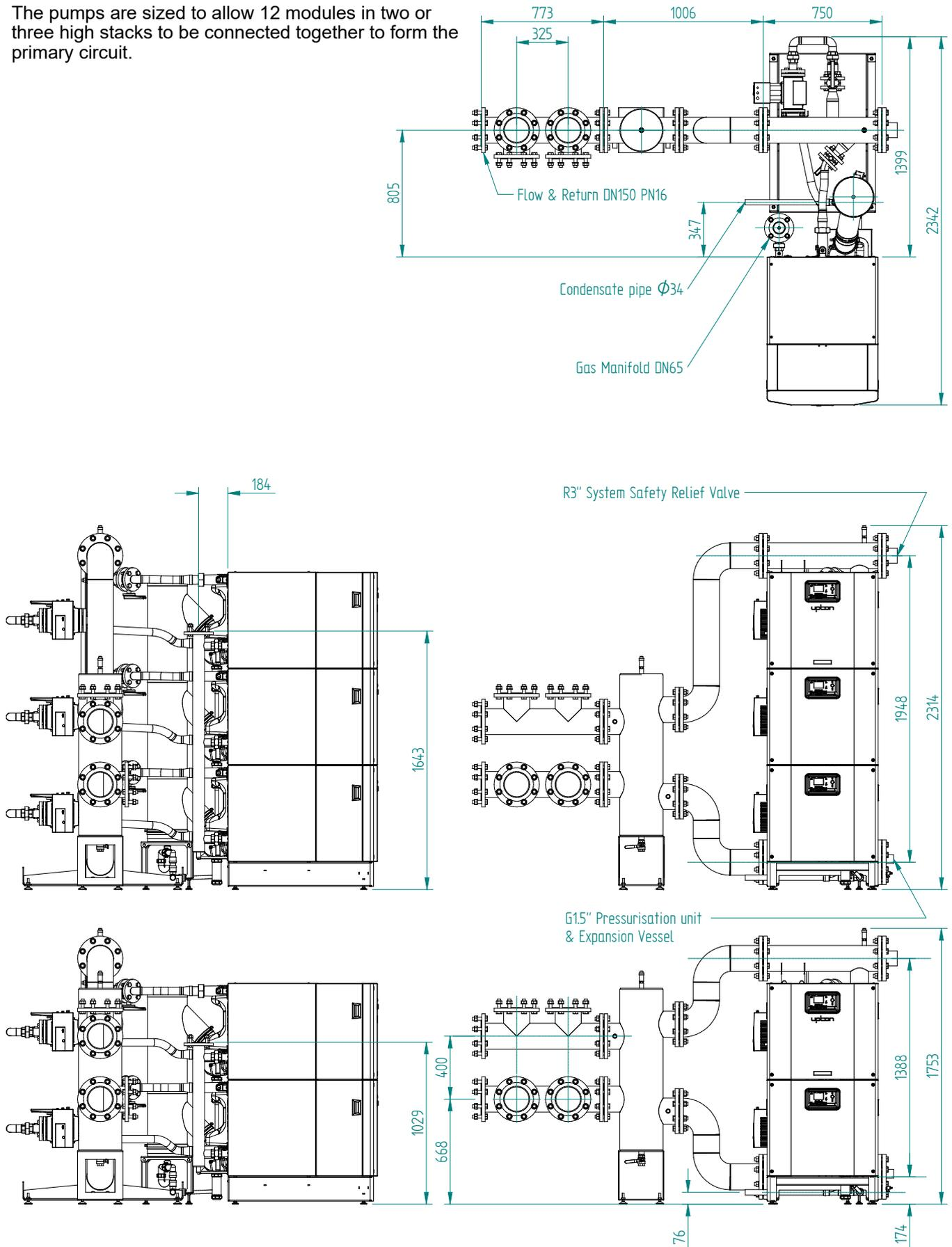
Figure 3.2.3 – UF200 & UF250 3MW Primary circuit and Gas manifold pipe kit
