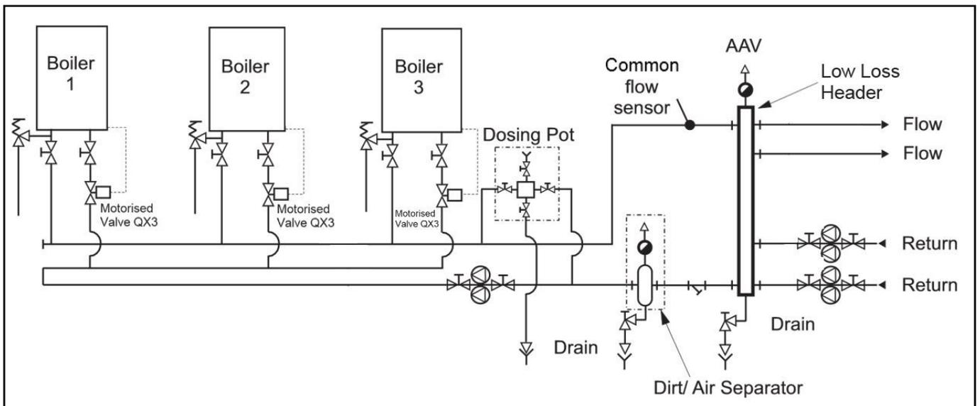
**Figure E 1.3.6 - Schematic 6 - Reverse Return Primary Circuit with Individual Motorised Boiler Isolation**
