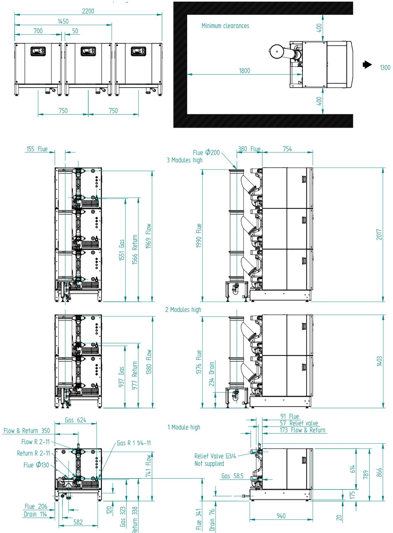
Figure 3.1.1 - Dimensions and Clearances UF100 & 150
