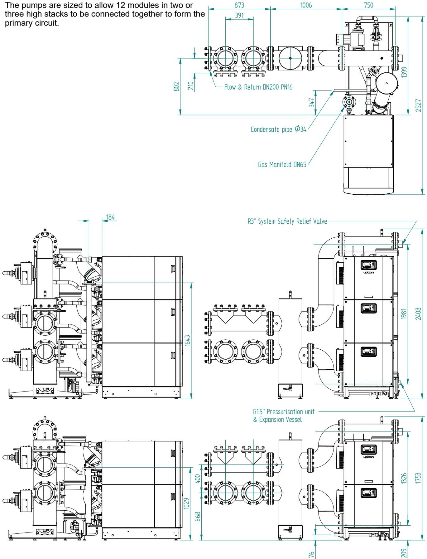
Figure 3.2.5 – UF300 & UF350 4MW Primary circuit and Gas manifold pipe kit
