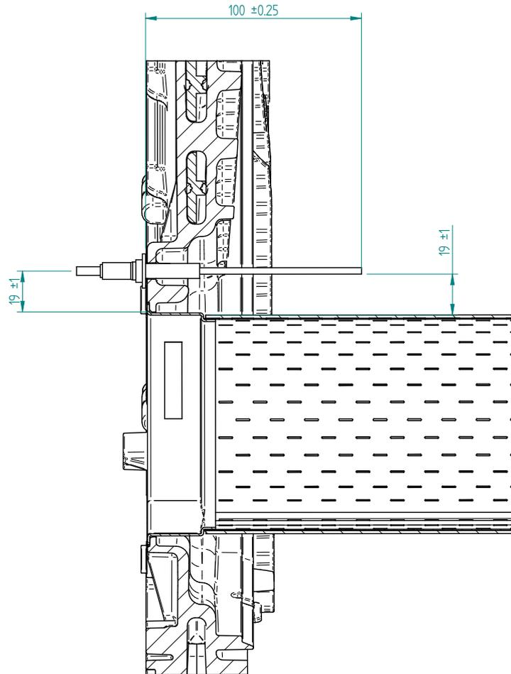
Figure 10.2.2 - Flame Probe position
