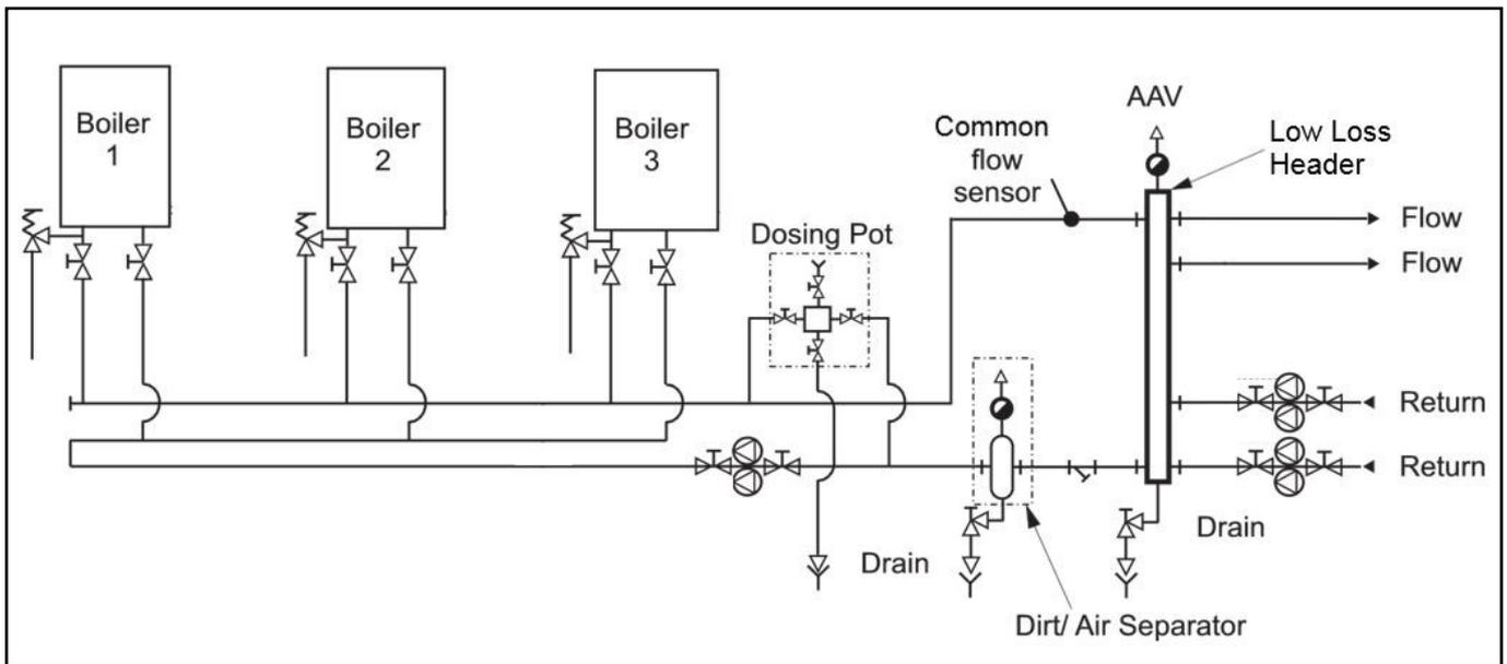
**Figure E 1.3.4 - Schematic 4 - Reverse Return Primary Circuit**
