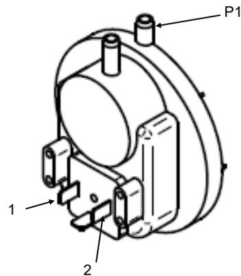
Figure 11.11 Air pressure switch
