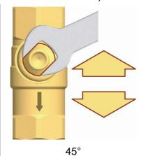
Ball valve half-closed, flow in both directions.
