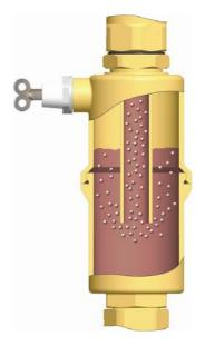
The air liberated from the solar fluid is collected in the upper part of the Airstop and can be released at the vent plug.
