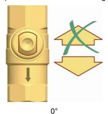
Ball valve open, flow only in flow direction.
