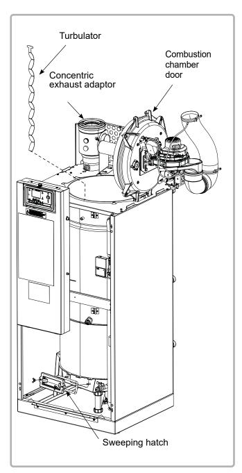
figure 20 - Cleaning the combustion chamber/exchanger
