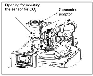
figure 15 - Measurement orifice
