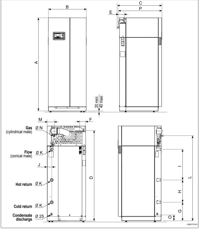
figure 1 - Dimensional characteristics
