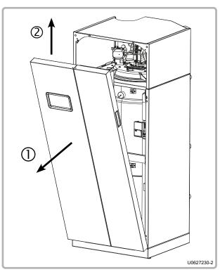
1. Tilt the front panel forward (use the handles located on the door thickness).
