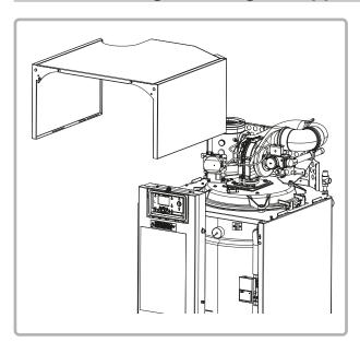
figure 4 - Removing the upper cover
