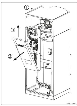
figure 16 - Access to the control panel
