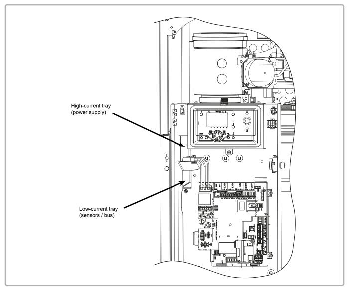
figure 18 - Electrical cable duct
