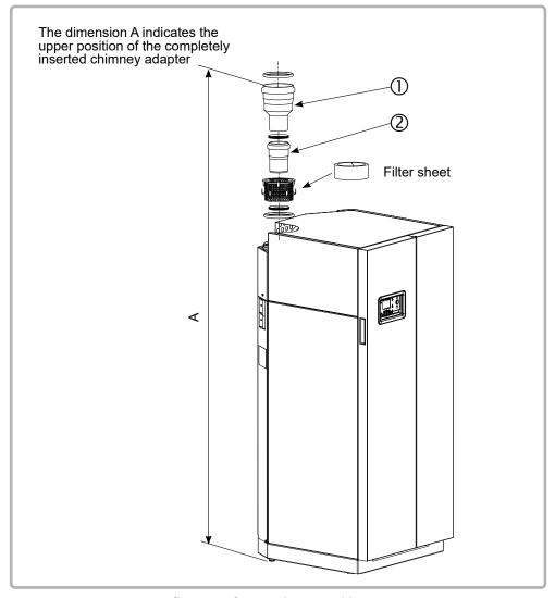
figure 5 - Connection to a chimney
