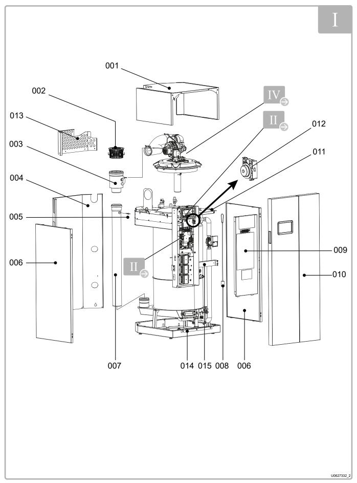
figure 29 - Casing/insulation
