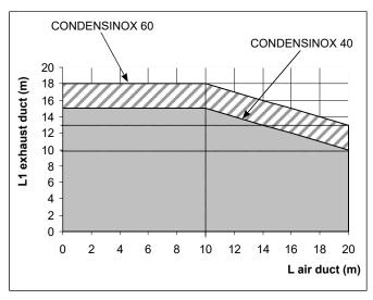
figure 9 - Max length of C53 type ducts
