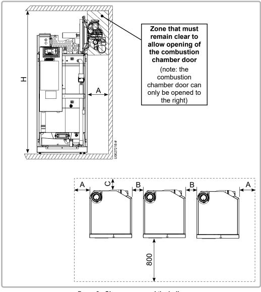
figure 2 - Clearance around the boiler
