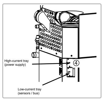
figure 17 - Electrical cable duct
