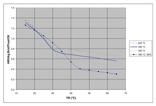
Recuperator power output per kg of fuel oil for different flue gas inlet temperatures and recuperator return temperatures TR at boiler nominal loads as well as 50% load (for 180°C nominal inlet temperature)
