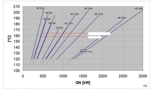
Flue gas temperature diagram Melbury HE, fuel oil with clean boiler
