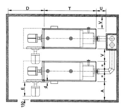
It must be possible to open the furnace door, including burner, by 90°.
