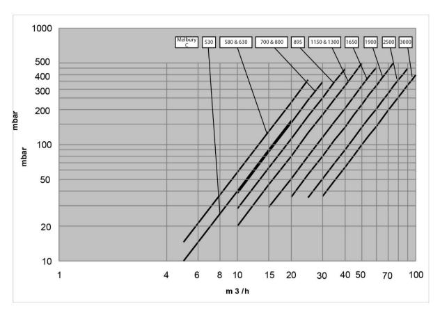
Pressure resistance in relation to water flow of the recuperators Melbury C
