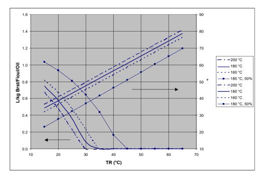
Condensate amount per kg of fuel oil and flue gas temperatures for different flue gas inlet temperatures and recuperator return temperatures TR at boiler nominal loads as well as 50% load (for 180°C nominal inlet temperature)
