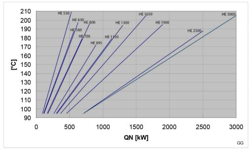
Flue gas temperature diagram Melbury HE, natural gas with clean boiler
