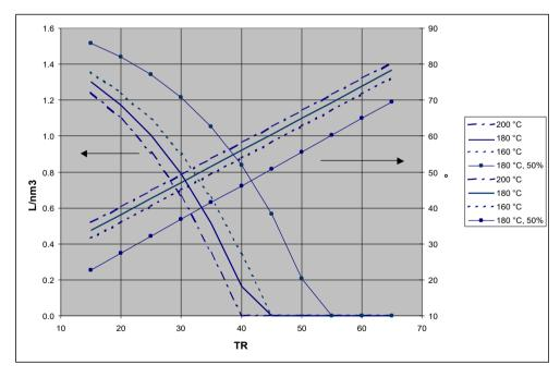
Condensate amount per nm3 of gas and flue gas temperatures for different flue gas inlet temperatures and recuperator return temperatures TR at boiler nominal loads as well as 50% load (for  $180^{\circ}$ C nominal inlet temperature)
