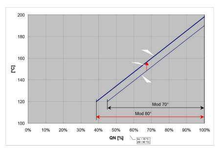
Flue gas temperature – Boiler power diagram, example for two average boiler water temperatures
