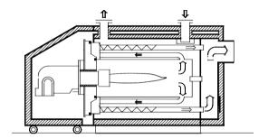
The third pass is equipped with turbulators. Their turbulent action further increases the heat exchange and allows the system to work at low combustion gas temperatures, guaranteeing optimal fuel use as a result.
